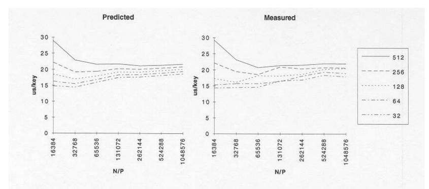
Figure 1.12 Estimated and measured execution time of parallel sample sort on the CM-5.
