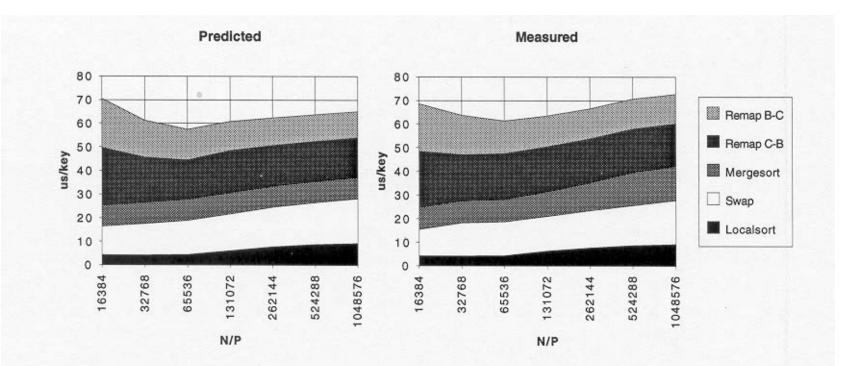
Figure 1.5 Predicted and measured execution times per key on 512 processors for the phases of bitonic sort. The time for the single gather is included in the time for the remap from a blocked to a cyclic layout; likewise, the time for the scatter is included in the time for the remap from a cyclic to a blocked layout.
