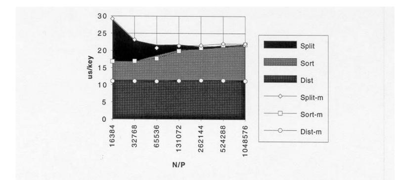
Figure 1.13 Estimated and measured execution times of various phase of parallel sample sort on 512 processors.
