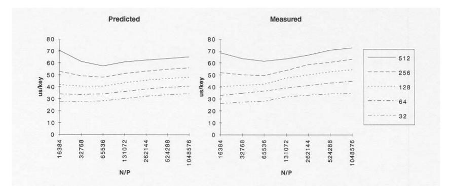
Figure 1.4 Predicted and measured execution time per key of bitonic sort on the CM-5. Times are shown to sort between 16K and 1M keys per processor on 32, 64, 128, 256 and 512 processors.
