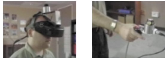
Figure 5. The HiBall being used by Kevin Arthur to track the head and hand for the presence experiments in [22].
