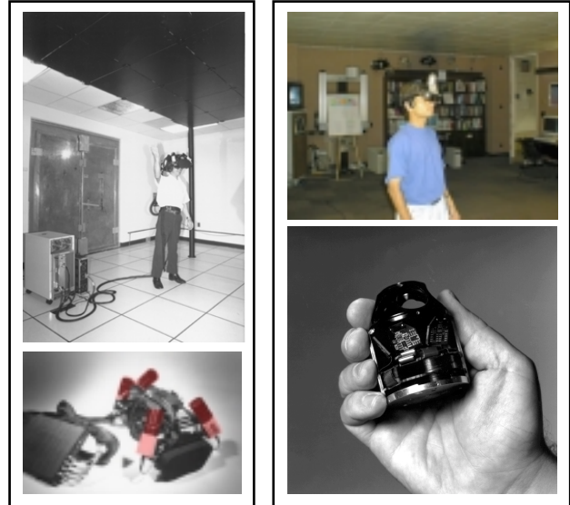
Figure 1. Left: the original UNC optoelectronic ceiling tracker in use, and a close-up of the head-mounted display and sensor fixture, along with the signal processing and communications electronics pack. Right: the new system in use, and a close-up of the self-contained HiBall with lenses and part of the cover removed. See also the color plate Welch 1.
