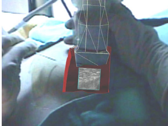
Figure 1: A typical physician's view of an augmented reality breast needle biopsy guidance system. The physician holds the ultrasound probe with her right hand. The captured ultrasound image is displayed at the 3 dimensionally correct position inside the patient's breast. The "pit" (the red square hole) serves as a virtual window opened on the patient's skin surface. The ultrasound slice, the pit, and the wireframe outline of the ultrasound slice are rendered with the 3D computer graphics technique. The rest of image is captured by a camera mounted on the physician's head.
