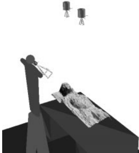
Figure 3.1: A sample environment for which the proposed tracking system is well-suited. In this application, a physician examines a patient lying on the table using AR visualization. The region of interest is small, the lighting under control, and the viewpoints and view directions for which computer-augmented images will be needed are determined by the physician's reach and by the surgical field.
