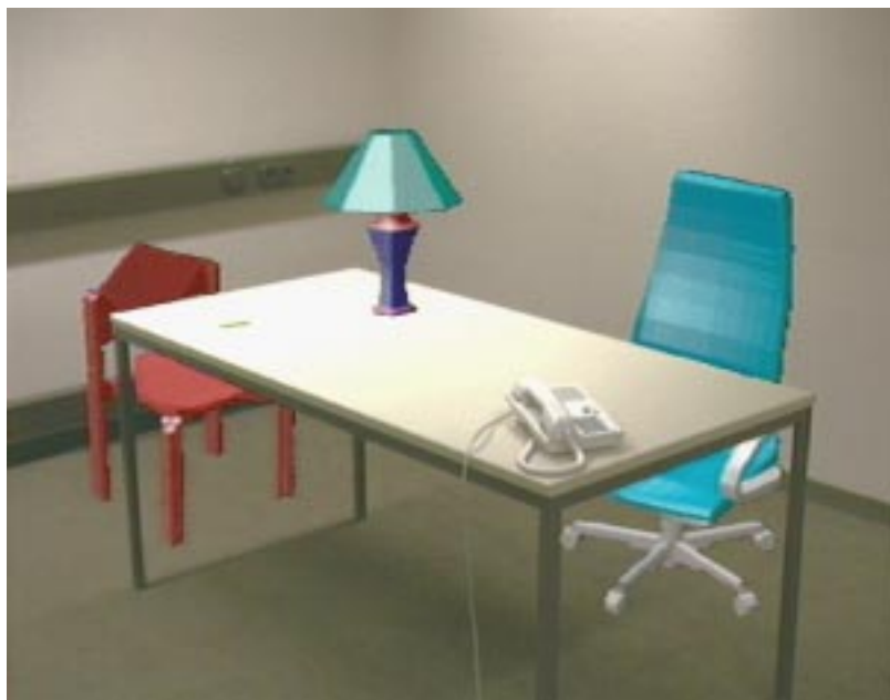
Figure 1.1: A simple AR environment. The walls, floor, table, and telephone are all real objects. The two chairs and the lamp on the table are all synthetic. Note how the lamp is aligned with the table top; it neither floats above the table nor sinks into the table. Also note that the synthetic lamp occludes part of the real table, while the real table occludes the two synthetic chairs. These two tasks are frequently difficult to perform in AR systems. Image ©1995 David Breen, Eric Rose, European Community Research Center.
