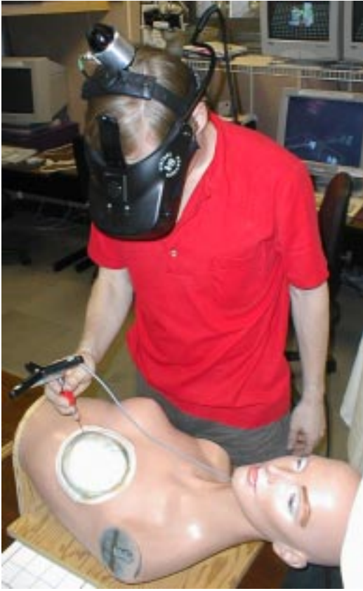
Figure 4.1: ( left ) A re-creation of the scene of the user experiment. The user wears an HMD that lacks see-through capability. The user inserts a tracked needle into a target within the medical phantom in the mannequin torso. The location of the target and the needle were both depicted in the virtual world presented to the user (Figure 4.2).
