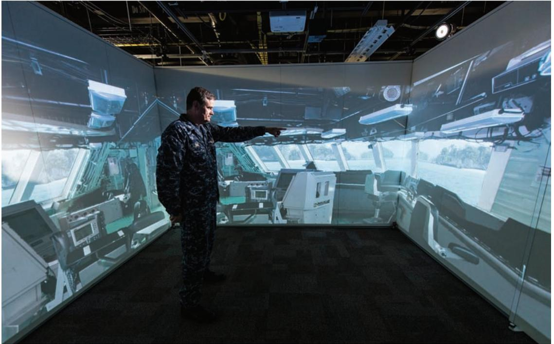
**Figure 4.** HuSIS interaction space. This central experiment space is structured to support various input and output capabilities, including CAVE-like spatial augmented reality (SAR) and head-worn display experiences. Here we show a US Navy sailor visualizing the bridge of the USS Freedom, a littoral combat ship.
