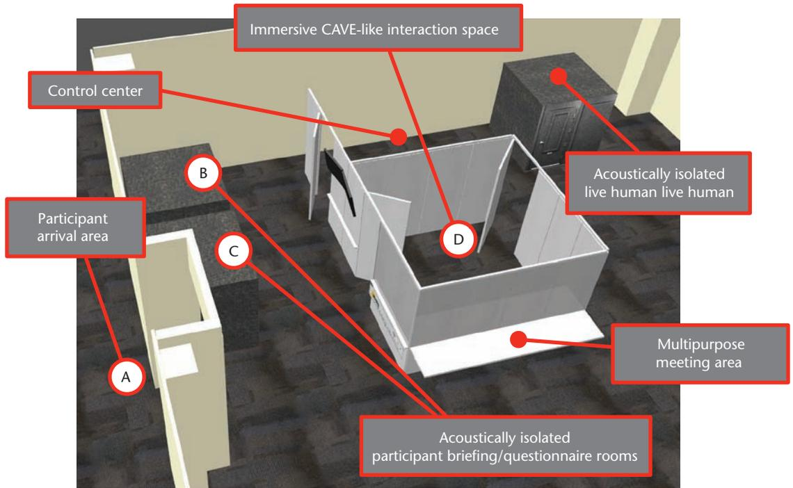
**Figure 1. Layout of the Human-Surrogate Interaction Space (HuSIS) in a corner of our existing lab space. The HuSIS system consists of areas designed to facilitate participant pipelining throughput and minimize unintentional influences on the participant’s mindset and perceptions and on the context surrounding the interaction. Multiple participants can be moved through areas A through D, while the researchers operate (out of sight) in the live interactor room and control center.**
