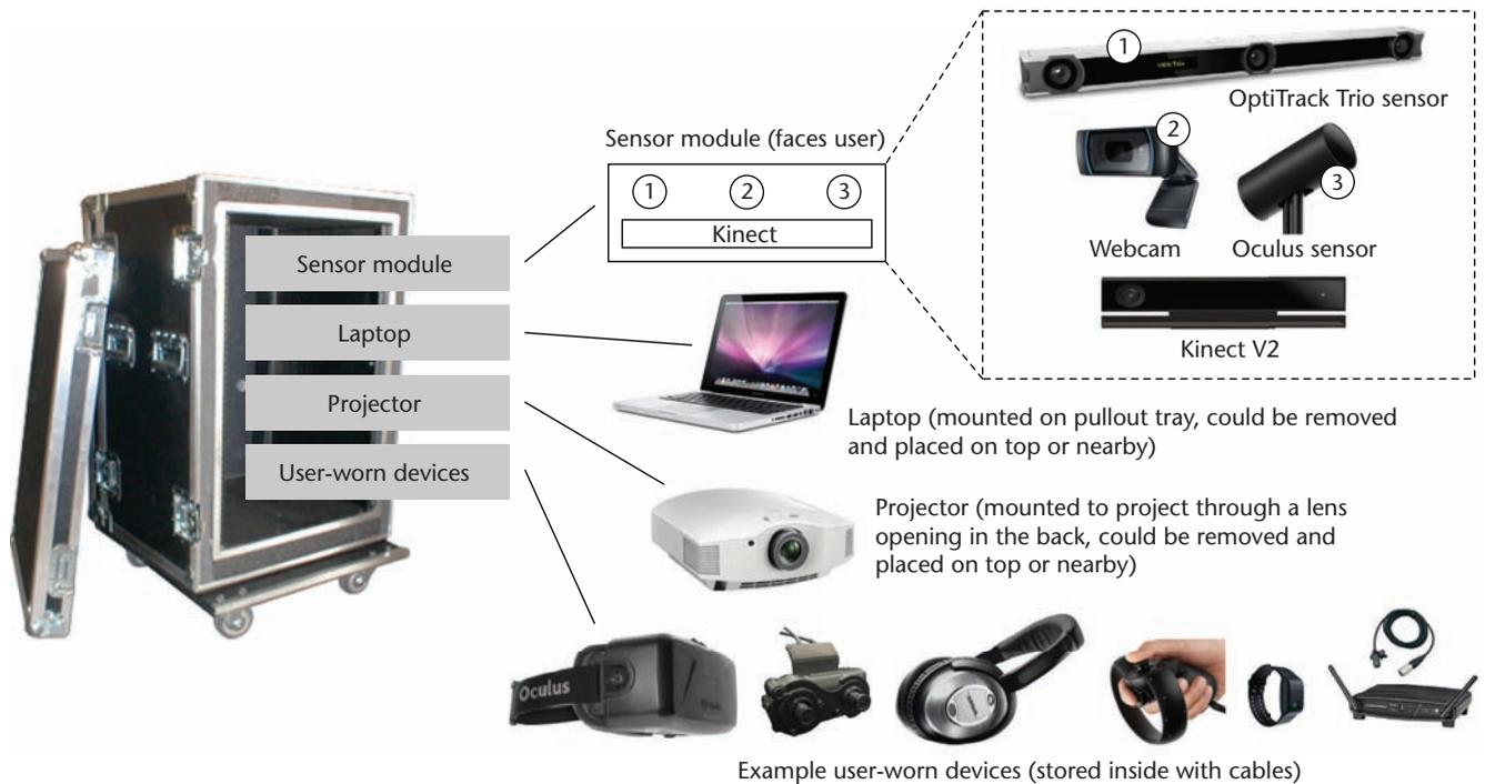
**Figure 7. A Transportable Human Surrogate Interaction System (THuSIS) unit. An Office of Naval Research (ONR) Defense University Research Instrumentation Program (DURIP) grant is supporting the development of six such units, which could be used together in one location or independently in separate locations to increase their effectiveness and impact.**
