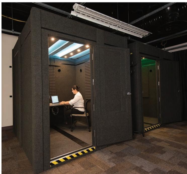
Figure 3. Acoustically isolated participant isolation rooms. These two rooms allow researchers to nearly double the experimental rate when including pre/post briefings and questionnaires.
