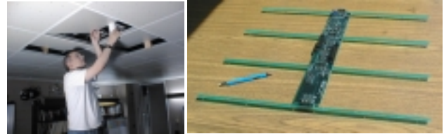
Figure 3. Left: Bishop lifts some Ceiling panels. Right: an individual Ceiling panel module showing the main PC board with four LED strips (eight LEDs per strip).
