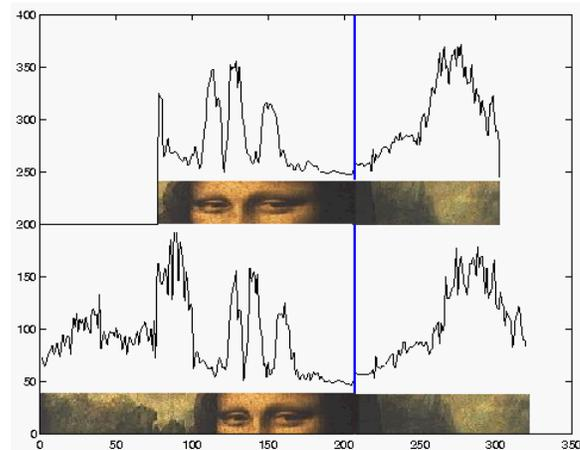
**Figure 4:** The intensity profile of a single scan line through the eyes compares the original projected image (bottom) to the warped version seen by the camera. The blue line locates the crease in the walls of the display surface.
