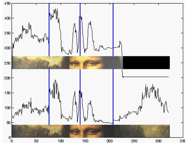
**Figure 6:** The intensity profile of a single scan line through the eyes compares the original projected image (bottom) to the version seen by the camera *after* the correct warp is found. Thus a correct solution means that the intensity profiles match: the camera captures an image exactly like the original. The correct pre-projection warp compensates depth-based distortion. The blue line locates corresponding image features.
