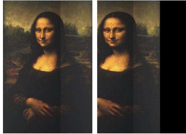
**Figure 3:** The left image is the projected image as viewed through the lens of the projector. The right image is the sensed image detected by the camera. Note the lateral warping that the display surface induces on the image seen by the camera. The eyes are 30% farther apart as a result of the projective warping caused by the tilted display surface.
