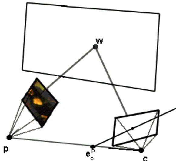
**Figure 1:** Epipolar geometry of the problem. A projector at position  $p$  generates a controlled image onto a surface of unknown shape. The known relative geometry of the camera and projector allows for the computation of epipolar lines in camera  $c$ , for each projection ray that intersects the world. The image of  $w$  as sensed at  $c$  must lie along the epipolar line.
