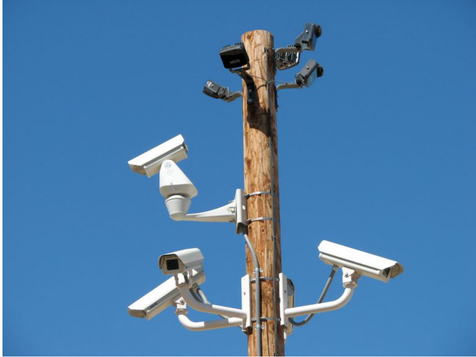
Figure 1.4: Light pole with sensors at Camp Pendleton, CA. The bottom 3 cameras are fixed. The camera in the middle is an active camera. Other sensors are placed on top. Image by Dr. Amela Sadagic.
