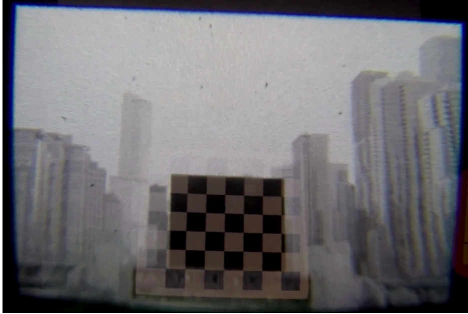
Figure 4.3: A sample frame using our latency compensation algorithm under fast panning motion ( 50^\circ/\text{s} ) where the majority of the field of view is dominated by a off-kilter grayscale planar image of a city skyline, in which a small cutout region is registered to the physical checkerboard. Note that the cutout and the checkerboard interior are well aligned and details in the city photo are visible.
