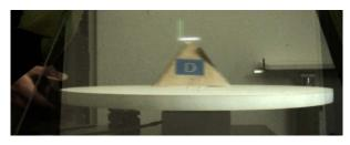
(a) Conventional 60 Hz color display. Note that the overlay is displaced significantly from the tip of the pyramid.
