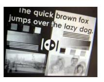
(b) Projected using a conventional grayscale DMD projector. Note that the image is generally sharp within each consecutive frame, though these two frames are distinctly visible, which results in jumpy motion.
