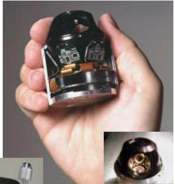
The HiBall technology is packaged in a golf-ball sized device fitted with specialized optical sensors and lenses that can be head-mounted to track the user's view perspective through a virtual or augmented reality scene. Housed inside the device are stacked, folded, flexible PC boards.
