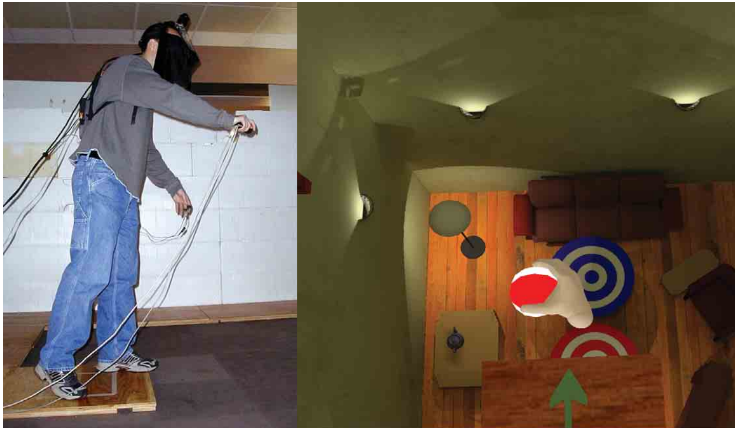
Figure 1. (left) A user stands on a wooden ledge (passive haptics) corresponding to the ledge in the VE; wires go to the video source, tracker, wand, and physiological measuring devices. (right) The user's view into the pit; the avatar of the user's hand is visible as he prepares to drop the red-and-white ball on the target below (University of North Carolina at Chapel Hill, inspired by Mel Slater, University College London).
