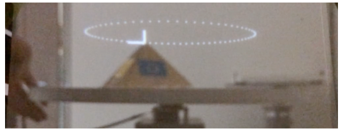
(b) Experimental display at 1 kHz. Without the need to operate at the maximum rate of 22727 Hz, 1 kHz is enough to show the benefit of using this low latency display.
