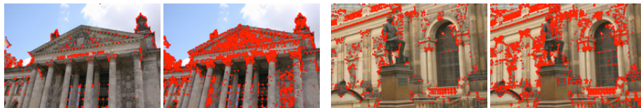
Fig. 4. This figure shows the distribution of keypoints (for two datasets) from the Harris (left image in the pair) and FAST (right image in the pair) corner detectors. The FAST detector not only detects more keypoints, but has a higher entropy for its detections.
