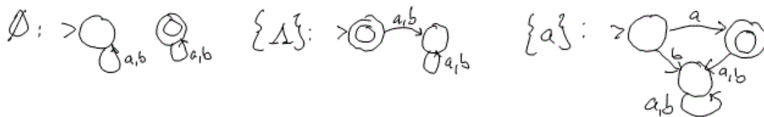
Figure 12.4: Machines with \Sigma = \{a, b\} that accept base case languages \emptyset , \{\Lambda\} , and \{a\} . The machine for \{b\} , similar to the machine for \{a\} , would complete the set of base cases.
