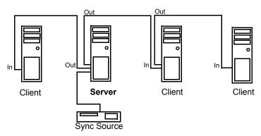
Figure 2.2 Example of Frame Lock Hardware Connections
