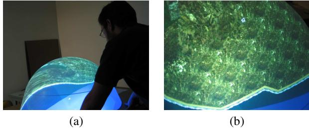
Figure 4: Results of the rendering algorithm. (a) A user inspects a 3D terrain of a coastline region. (b) A view of the model captured from the same view of the user shown in (a). The image is composed of three of the six overlapping projectors.
