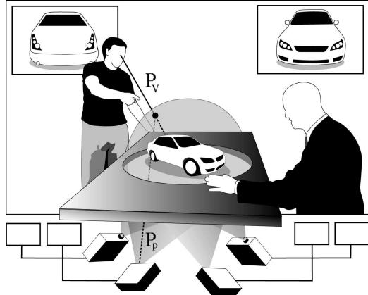
Figure 1: A conceptual drawing of the DOME. A back-projection screen is shaped into a curved surface to provide simultaneous viewing for the users. Once calibrated, projectors and rendering PCs cooperatively render distinct images for both viewers.
