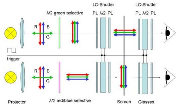
Figure 2: Filter principle for left and right eye. The projector is on the left and the users eye on the right.
