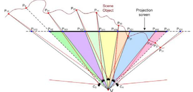
Figure 6. The projection screen sub-image is composed by the overlapping areas and the non-overlapping areas. They depend on the scene objects' depth.
