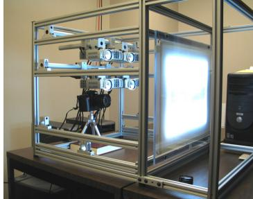
Figure 1: A four-projector prototype of a light field display.
