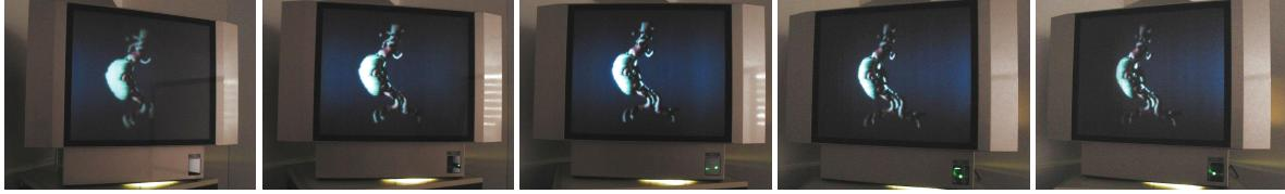
**Figure 2. Holographic display example. The images that were taken from different positions in front of the display. The 3D model is an abdominal aortic aneurysm reconstructed from CT data.**
