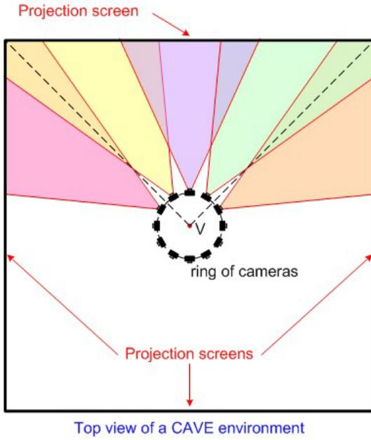
Figure 5. Reprojection of images from the ring of cameras to the projection screens of a CAVE.
