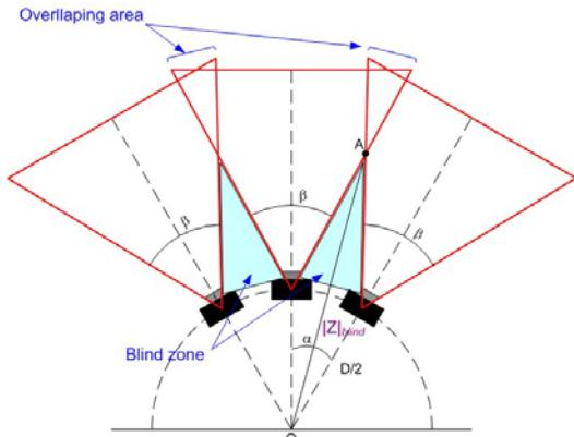
Figure 3. Field-of-view of cameras at the ring and the blind zone between adjacent cameras .
