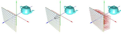
Figure 3: Parallel rays in a microlens array. (**Left**) A teapot scene is to be visualized. (**Middle**) A traditional way to render MCOP images is to render the perspective view for each screenlet one by one. (**Right**) Our novel rendering algorithm renders groups of parallel rays, significantly reducing the number of rendering passes needed.
