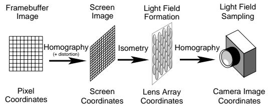
Figure 2: Elements involved in display calibration and the associated coordinate systems.
