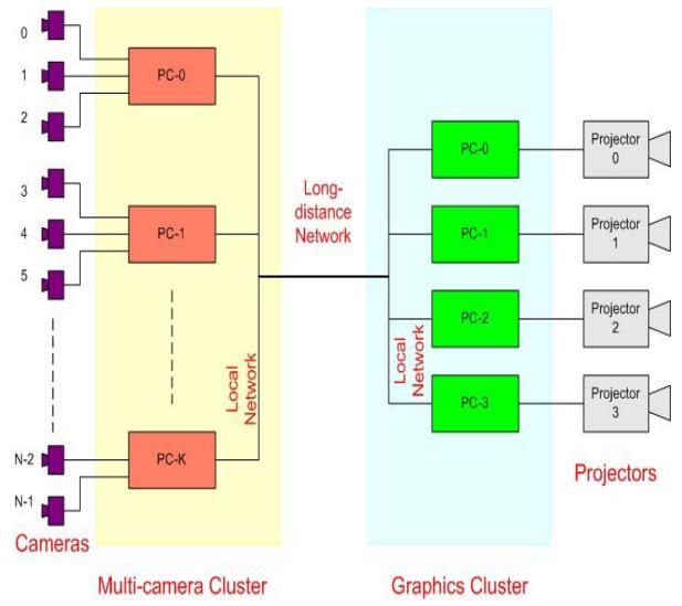
Figure 1. Block diagram of the panoramic tele-immersion system.
