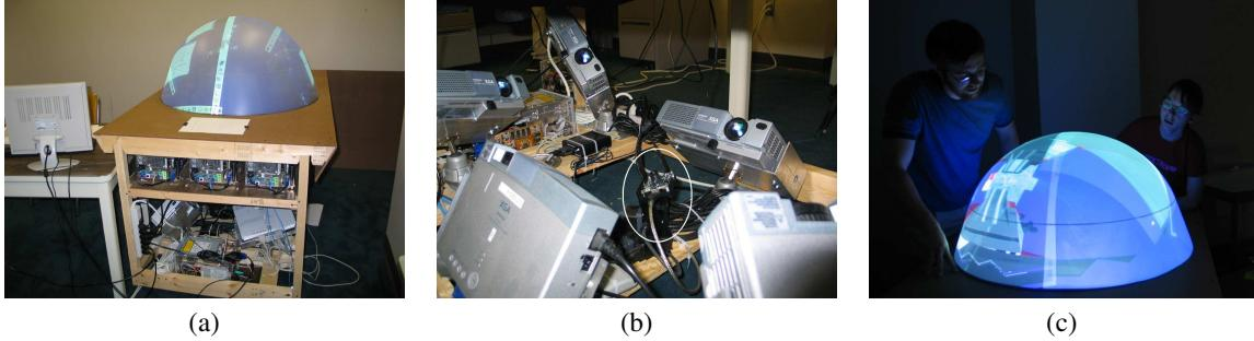
Figure 2: Three views of the DOME prototype display. (a) A view of the DOME from the side depicting the display surface shape, mounting cabinet, and projector/computer array. (b) A view of projectors and a camera is mounted beneath the display surface. The camera is attached to a pan-tilt unit to support calibration of the display across a wider field of view (circled in white for clarity).
