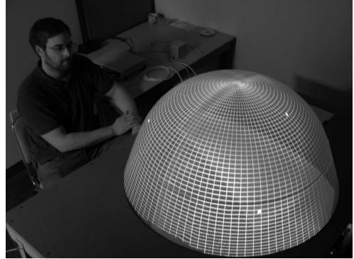
Figure 3: Example calibration results. An image of the DOME display after calibration and all rendering clients display coherent longitude-latitude lines.
