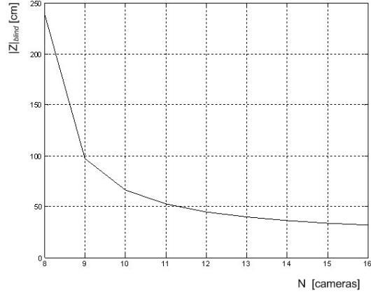
Figure 4. The blind distance  $|Z|_{blind}$  as a function of the number of cameras  $N$ , with  $\beta = 48.5^\circ$  and  $D = 35\text{cm}$ .
