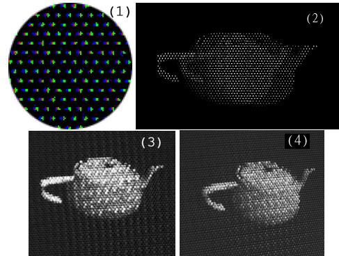
Figure 5: Preliminary view-dependent effect. (**1**) A close-up image of the visibility map from calibration. Different colors encode which pixel is visible in which view(s). (**2**) We rendered a stereo pair and merged them into a single image based on the visibility map. (**3, 4**) Right and left views of the composite image from two calibrated viewpoints.
