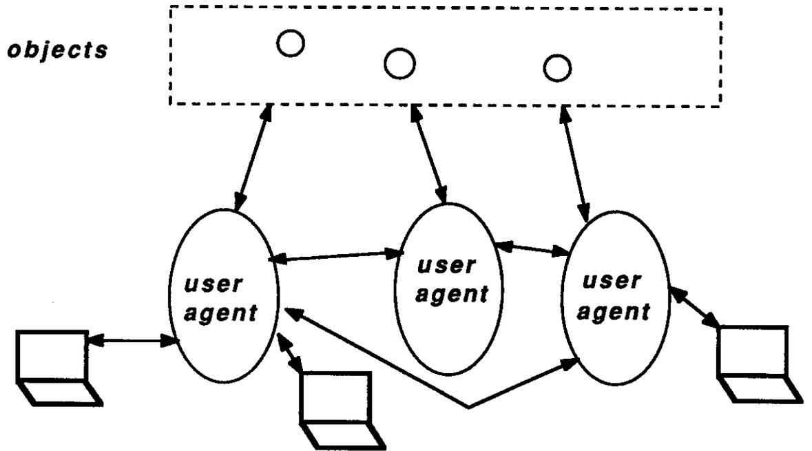
**Fig. 2.2 Multi-User Tool (Decentralized Control)**
