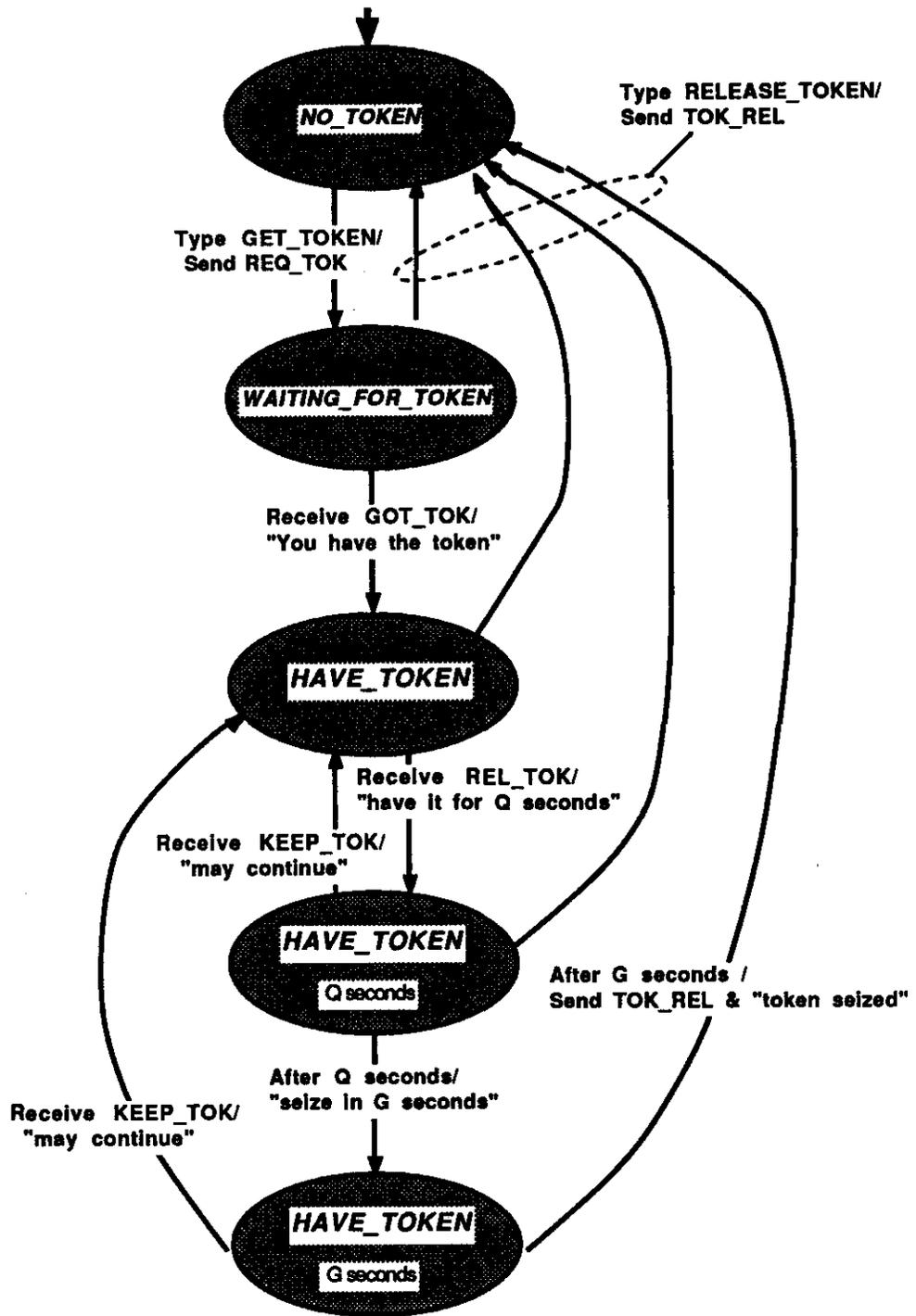
**Fig. 2.5 Token Control States for User Process**
