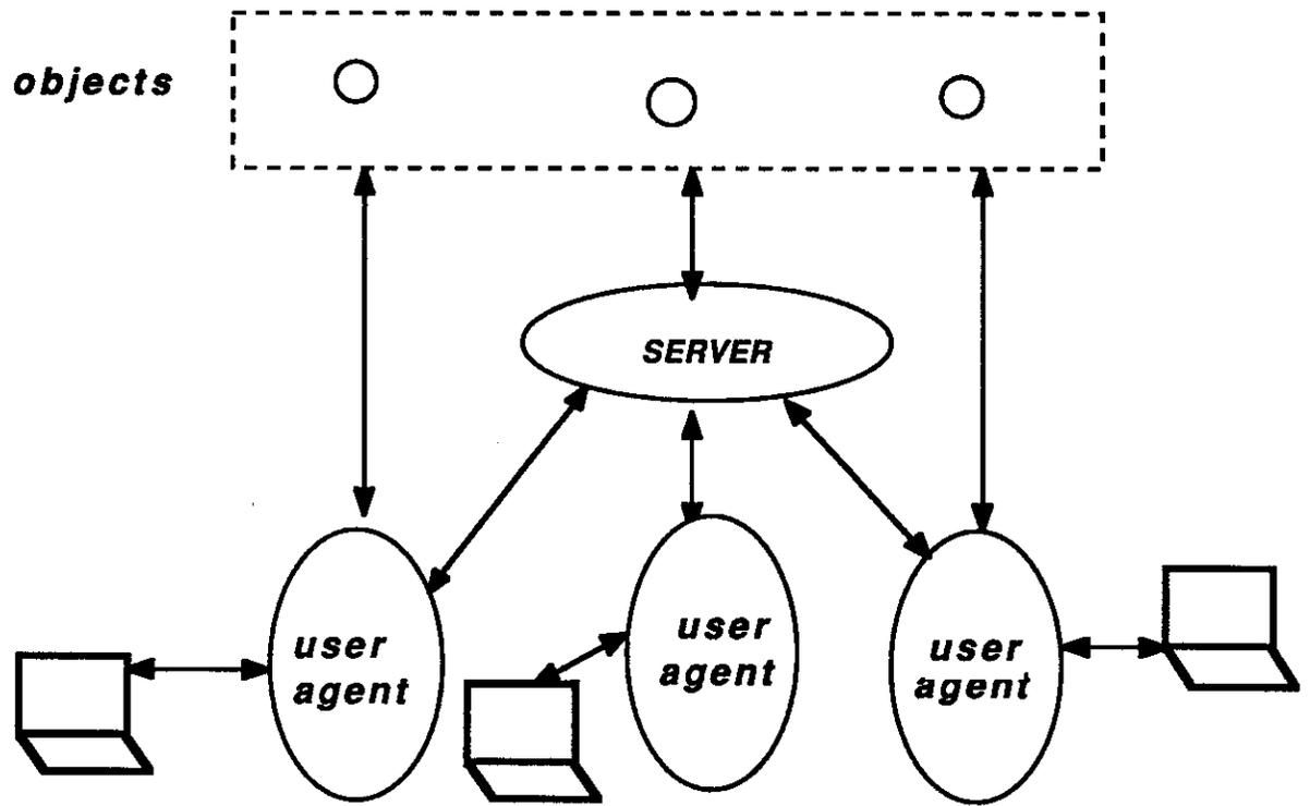
**Fig. 2.1 Multi-User Tool (Centralized Control)**
