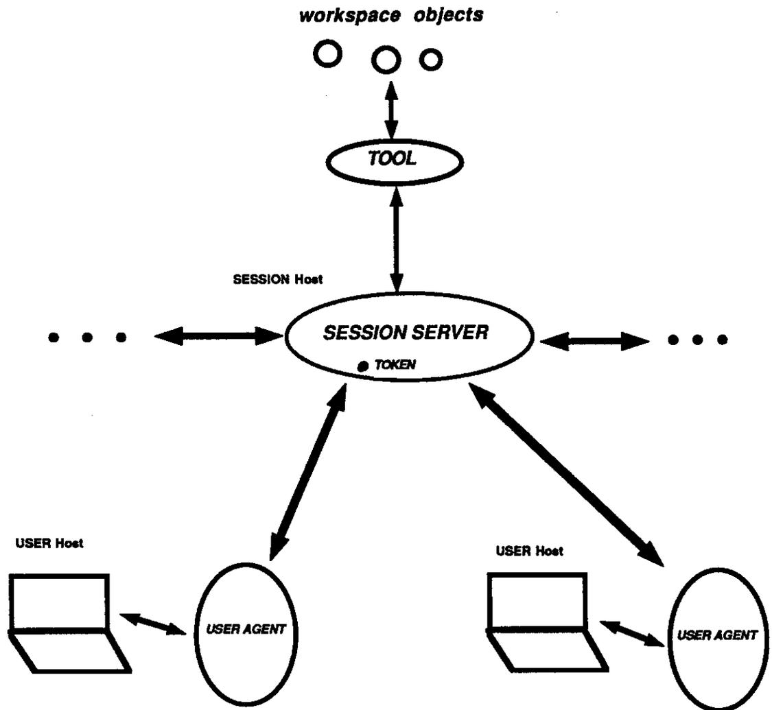
**Fig. 2.3** *Sharing a Single-User Tool in a Real-Time User Cooperation*
