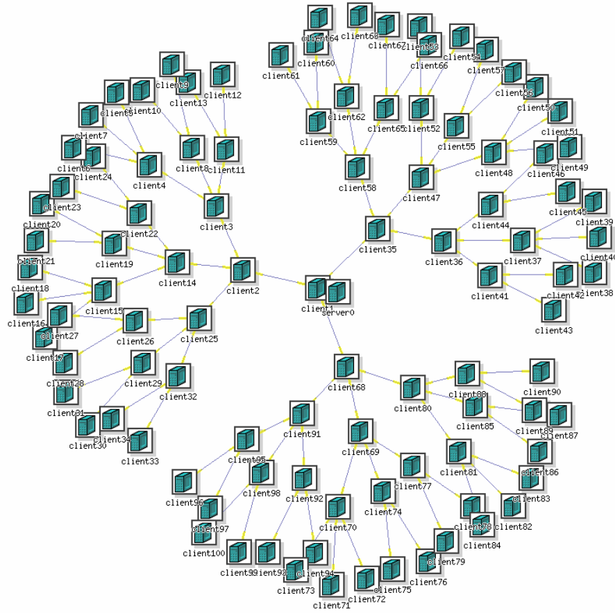
Figure 6.5: An experiment topology with 60 clients is depicted in this image taken from the Emulab testbed’s web interface. This topology, even though it uses a tertiary tree for efficiency, nearly surpasses Emulab’s resources by requiring 131 PCs to be provisioned.
