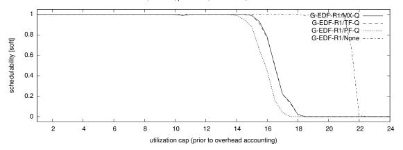
Figure 7.14: SRT schedulability under G-EDF-R1 scheduling with  $n_r = 24$ , pacc = 0.1, and wratio = 0.75 assuming light exponential utilizations, moderate periods, and short critical sections. The curves corresponding to MX-Q and TF-Q locks overlap.
