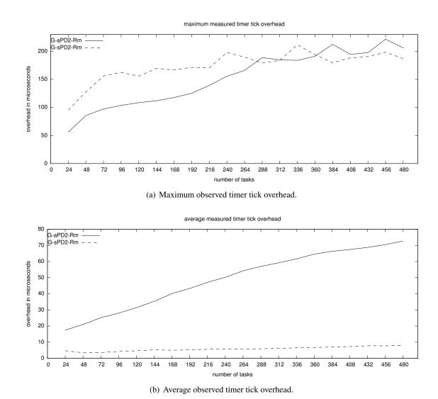
Figure 4.9: Timer tick overhead under  $G-aPD^2-Rm$  and  $G-sPD^2-Rm$ . Quantum staggering is effective and lowering average-case overheads, but does not lower worst-case overheads.
