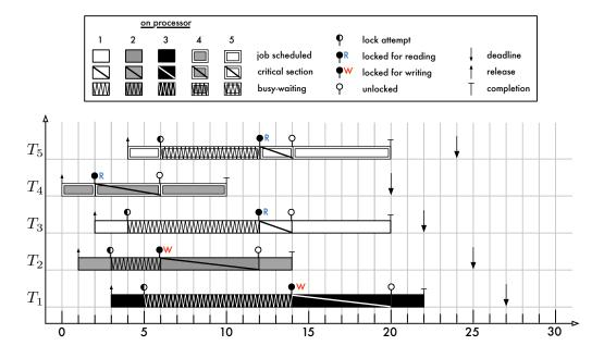
Figure 5.4: Example of reduced blocking under phase-fair locks. All readers meet their respective deadlines because they are not blocked by more than one write request (due to Property PF1). Note how the contending readers  $(J_3, J_4)$  yield to a writer  $(J_2)$  at time 4, which is followed in turn by a writer  $(J_1)$  yielding to the aforementioned readers: this exemplifies the "after-you politeness" implicitly required by the definition of phase-fairness.
