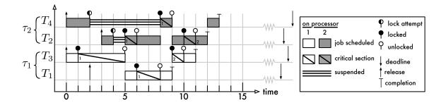
Figure 2.39: Example MPCP schedule for the same scenario as shown in both Figure 2.36 and Figure 2.38. The schedule is discussed in Example 2.19.
