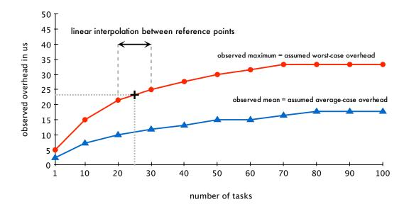
Figure 4.2: Illustration of an overhead model. Worst-case and average-case overheads are modeled as a piece-wise linear function of the task set size n. The reference points are the observed maximum and mean overheads for the tested task set sizes, which are typically a multiple of m (in this example, m=10). An exception is n=1 since at least one task is required to collect overhead samples.
