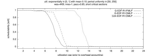
Figure 7.18: SRT schedulability under G-EDF-R1 scheduling with the global FMLP, G-EDF-R1 scheduling with the global OMLP, and C24-EDF-R1 scheduling with the clustered OMLP for light exponential utilizations, long periods,  $n_r = 1$ , pacc = 0.85 and short critical section lengths.
