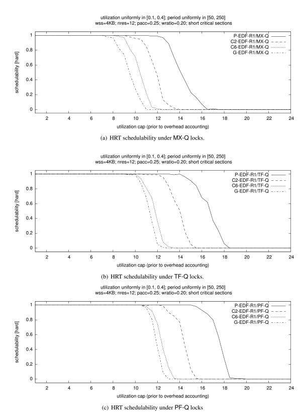
Figure 7.15: Graphs showing HRT schedulability under P-EDF-R1, C2-EDF-R1, C6-EDF-R1, and G-EDF-R1 scheduling with  $n_r=12,\ pacc=0.25,\ {\rm and}\ wratio=0.2$  assuming medium uniform utilizations, long periods, and short critical sections.
