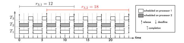
Figure 2.15: Devi's example of unbounded tardiness under G-FP scheduling with RM priorities (Devi, 2006). There are three tasks with parameters  $e_1 = e_2 = 2$ ,  $p_1 = p_2 = 3$ , and  $e_3 = 4$  and  $p_3 = 6$ . If all tasks release jobs periodically starting at time 0, all jobs of  $T_3$  miss their deadlines and exhibit unbounded tardiness. This is because  $u_3 = \frac{2}{3}$ , but  $T_3$  receives only an allocation of  $\frac{1}{3}$  on average.
