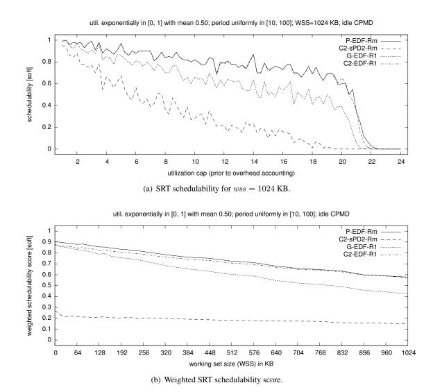
Figure 4.31: Graphs showing (a) SRT schedulability and (b) weighted SRT schedulability score of Comparison of P-EDF-Rm, C2-EDF-R1, G-EDF-R1, and C2-sPD<sup>2</sup>-Rm in terms of SRT schedulability for exponential heavy utilizations and moderate periods.
