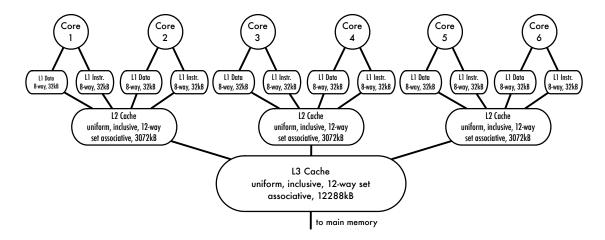
Figure 2.6: Illustration of the cache hierarchy of one chip of the experimental platform used in Chapters 4 and 7. The system contains four chips, for a total of 24 cores.
