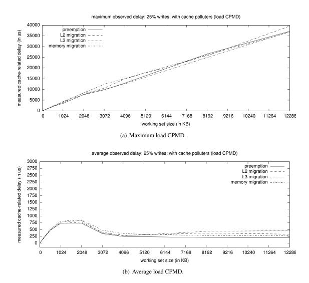
Figure 4.17: Graphs showing (a) maximum observed CPMD and (b) average observed CPMD as determined by the synthetic method in the presence of m cache-polluting background tasks. Note that inset (a) is plotted using a different y-axis scale due to the magnitude of the measured CPMD.
