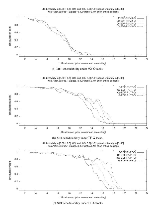
Figure 7.16: Graphs showing SRT schedulability under P-EDF-R1, C2-EDF-R1, C6-EDF-R1, and G-EDF-R1 scheduling with  $n_r = 12$ , pacc = 0.4, and wratio = 0.1 assuming light bimodal utilizations, short periods, and short critical sections.
