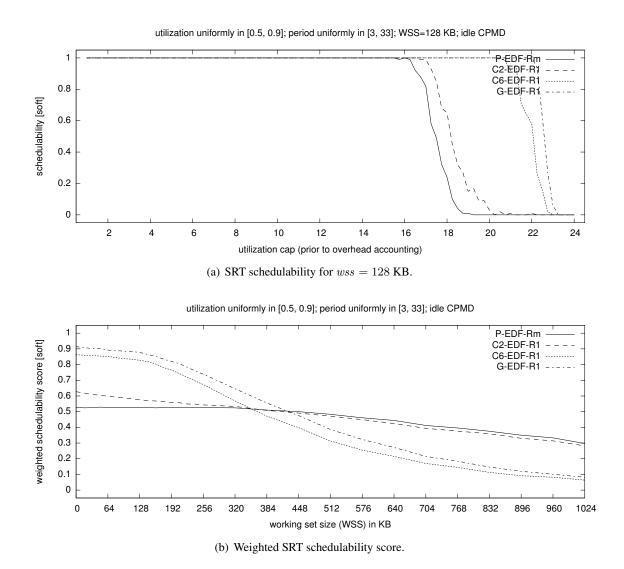
Figure 4.26: Graphs showing (a) SRT schedulability and (b) weighted SRT schedulability score of four EDF-based schedulers with different cluster sizes for uniform heavy utilizations and short periods.
