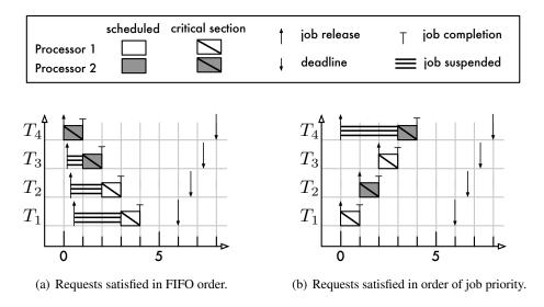
Figure 6.10: G-EDF schedules of n=4 tasks sharing one resource  $\ell_1$  on m=2 processors. Each job requires  $\ell_1$  for the entirety of its computation. (a) If conflicting requests are satisfied in FIFO order, then the job with the earliest deadline  $(J_1)$  may incur  $\Omega(n)$  pi-blocking if its request is issued just after all other requests. (b) If conflicting requests are satisfied in order of job priority, then a
