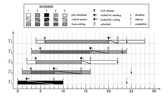
Figure 5.1: Example schedules of two writers  $(J_1, J_2)$  and three readers  $(J_3, J_4, J_5)$  sharing a resource  $\ell_1$  that is protected by a task-fair mutex lock. Jobs  $J_4$  and  $J_5$  miss their respective deadlines at times 23 and 24 due to the unnecessary sequencing of readers.
