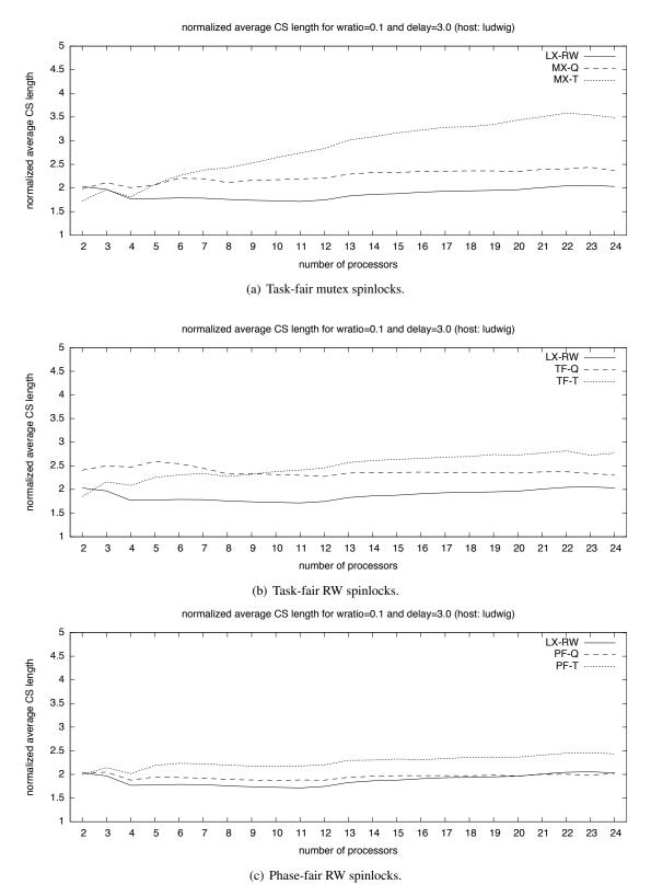
Figure 7.9: Average critical section length as a function of the number of contending processors, grouped by lock type with Linux as a baseline. See Table 7.2 for a list of the considered lock types.
