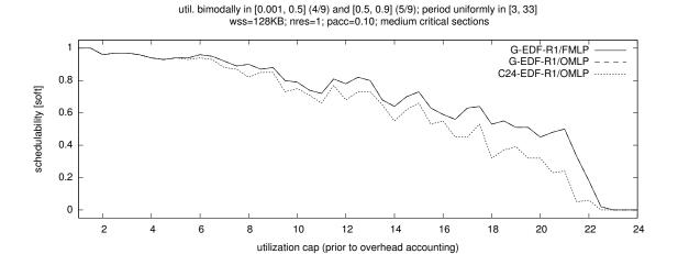
Figure 7.17: SRT schedulability under G-EDF-R1 scheduling with the global FMLP, G-EDF-R1 scheduling with the global OMLP, and C24-EDF-R1 scheduling with the clustered OMLP for heavy bimodal utilizations, short periods,  $n_r = 1$ , pacc = 0.1 and intermediate critical section lengths. The curves corresponding to global OMLP and the global FMLP overlap.
