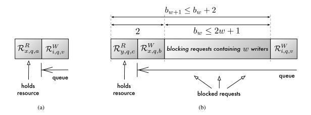
Figure 5.9: Illustration of Lemma 5.4 for the case  $N_{i,q}^W=1$  wherein a job  $J_i$  issues only one write request  $\mathcal{R}_{i,q,v}^W$ . (a) Base case w=0: at most one reader phase can block  $\mathcal{R}_{i,q,v}^W$ . (b) Induction step: allowing one additional write request  $\mathcal{R}_{x,q,b}^W$  can cause an additional reader phase to block  $J_i$  and hence increases the maximum number of blocking phases of either kind by at most two.
