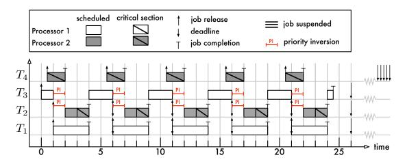
Figure 6.14: G-EDF example schedule of the task set  $\tau^{\phi}$  as given in Table 6.2 for m=2 and  $\phi=5$  assuming unrestricted priority boosting instead of priority inheritance.  $J_{3,1}$  still incurs  $\Omega(\phi)$  time units of s-aware pi-blocking. Unrestricted priority boosting is thus unsuitable for constructing locking protocols with O(n) maximum s-aware pi-blocking.
