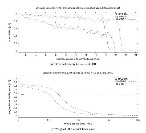
Figure 4.29: Graphs showing (a) SRT schedulability and (b) weighted SRT schedulability score of  $PD^2$ -based schedulers for uniform heavy utilizations and long periods.
