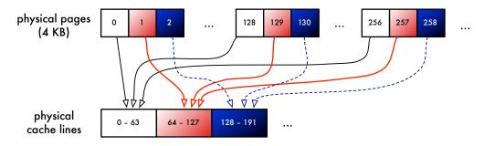
Figure 2.5: Illustration of page coloring. Physical pages are of the same page color if their contents map to the same physical cache lines. In this example, there are 128 distinct page colors (see Example 2.2).
