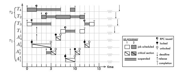
Figure 2.38: Example DPCP schedule for the same scenario as shown in Figure 2.36. There are four tasks  $T_1, \ldots, T_4$  assigned to m=2 processors sharing two resources  $\ell_1, \ell_2$  under P-FP scheduling. Both resources are local to processor 1; there are thus four agents,  $A_1^1, \ldots, A_1^4$ , assigned to processor 1. An agent is "released" when it receives an RPC request from a client job. The schedule is discussed in Example 2.18.
