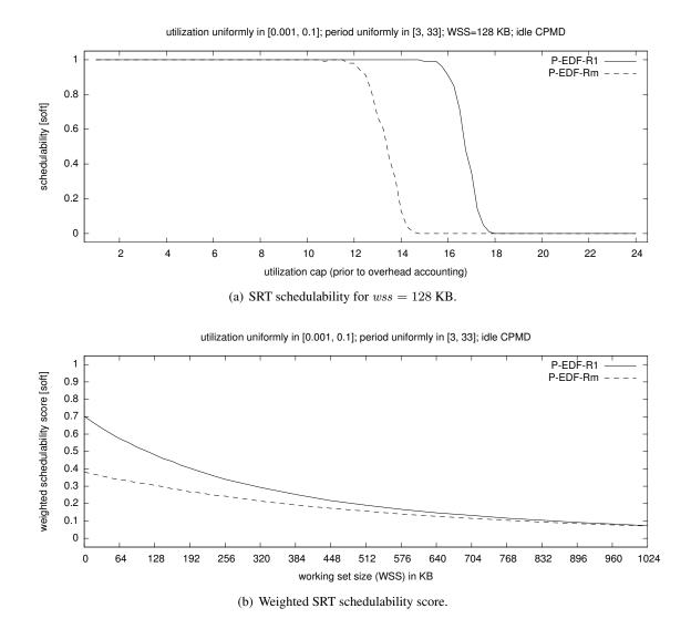
Figure 4.20: Graphs showing (a) SRT schedulability and (b) weighted SRT schedulability score of P-EDF-Rm and P-EDF-R1 for uniform light utilizations and short periods.
