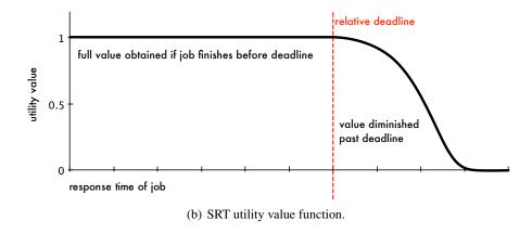
Figure 2.10: Illustration of HRT and SRT utility functions. In this example, there is no value in completing a late HRT job, whereas the utility of a late SRT job declines with increasing tardiness.
