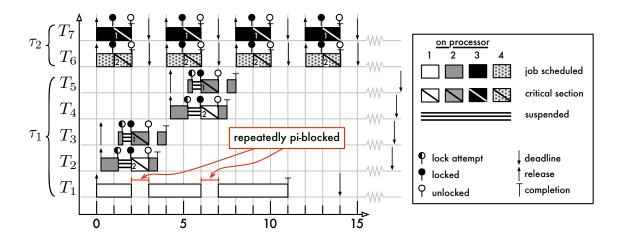
Figure 6.4: Example schedule of seven tasks sharing two resources  $(\ell_1,\ell_2)$  across two two-processor clusters under C-EDF scheduling. The digit within each critical section indicates which resource was requested. The example shows that priority boosting may cause jobs to incur pi-blocking repeatedly if c>1. If c=1, then lower-priority jobs cannot issue requests while higher-priority jobs execute and repeated pi-blocking due to priority boosting is not an issue.
