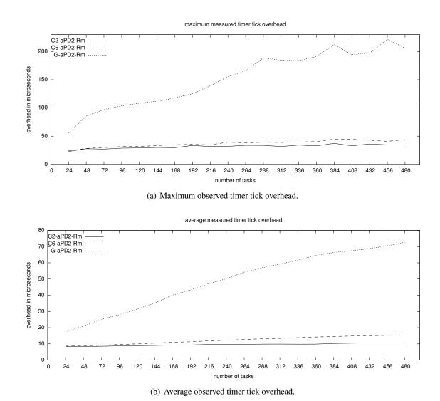
Figure 4.10: Timer tick overhead under C2-aPD<sup>2</sup>-Rm, C6-aPD<sup>2</sup>-Rm, and G-aPD<sup>2</sup>-Rm. Smaller cluster sizes result in lower maximum and average-case overheads.
