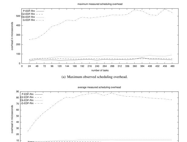
Figure 4.11: Scheduling overhead under P-EDF-Rm, C2-EDF-Rm, C6-EDF-Rm, and G-EDF-Rm. Smaller cluster sizes result in lower maximum and average-case scheduling overhead.
