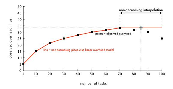
Figure 4.3: Illustration of forced monotonicity in the overhead model. While the observed overhead (either maximum or average values) exhibits a decreasing trend for  $n \ge 70$ , the overhead model uses piece-wise linear non-decreasing interpolation such that the resulting overhead model is monotonic.
