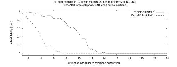
Figure 7.20: HRT schedulability under P-EDF with the clustered OMLP and under P-FP with the MPCP-VS for medium exponential utilizations, long periods,  $n_r = 24$ , pacc = 0.1 and short critical section lengths.
