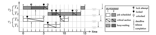
Figure 2.36: Example MSRP schedule. There are four tasks  $T_1, \ldots, T_4$  assigned to m=2 processors sharing two resources  $\ell_1, \ell_2$  under P-FP scheduling. The two resulting partitions are indicated as  $\tau_1$  and  $\tau_2$ . The digit within each critical section indicates which resource was requested.
