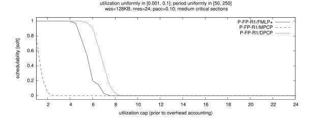
Figure 7.23: SRT schedulability under P-FP-R1 scheduling with the preemptive FMLP<sup>+</sup>, MPCP, and DPCP for light uniform utilizations, long periods,  $n_r = 24$ , pacc = 0.10 and intermediate critical section lengths.
