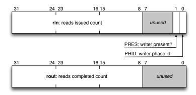
Figure 5.6: The allocation of bits in the reader entry counter and the reader exit counter of the PF-T algorithm (corresponding to line 2 of Listing 5.1).
