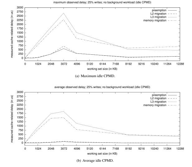
Figure 4.15: Graphs showing (a) maximum observed CPMD and (b) average observed CPMD as determined by the synthetic method in an otherwise idle system.
