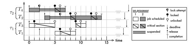
Figure 2.40: Example MPCP-VS schedule for the same scenario as shown in Figure 2.39. "Virtual spinning" occurs on processor 2:  $J_{2,1}$  executes during [3,4) while  $J_{4,1}$  waits, but when  $J_{2,1}$  requires  $\ell_1$ , it may not issue its request until  $J_{3,1}$  releases  $\ell_1$  at time 6.
