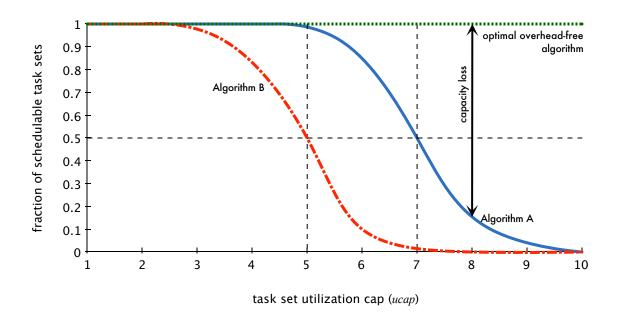
Figure 4.4: Illustration of a standard schedulability plot assuming m=10. Each curve depicts the ratio of schedulable task sets as a function of task set utilization, i.e., S(A,ucap) and S(B,ucap). In the absence of overheads, an optimal scheduler guarantees a schedulability of 1 until the total utilization exceeds m. Algorithmic and overhead-related capacity loss cause schedulability to gradually decrease in practice.
