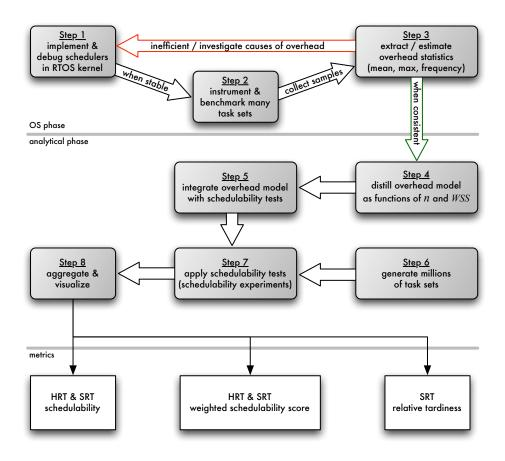
Figure 4.1: Flowchart illustrating the employed overhead-aware evaluation method.
