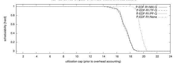
Figure 7.12: HRT schedulability under P-EDF-R1 scheduling with  $n_r = 24$ , pacc = 0.1, and wratio = 0.5 assuming medium uniform utilizations, long periods, and short critical sections. The curves corresponding to MX-Q, TF-Q, and PF-Q locks overlap.
