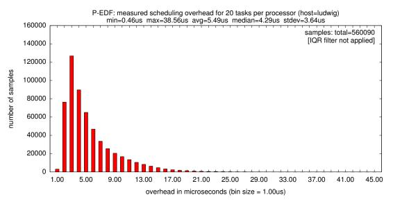
(b) Distribution of scheduling overhead samples for n = 480 (20 tasks per processor).
