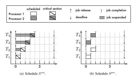
Figure 6.3: Illustration of Lemma 6.2 for n=4 and m=2 under P-EDF. Note that  $b_i \geq r_i^{seq} - r_i^{par}$ . For example,  $J_4$  incurs pi-blocking during [0,2) in  $S^{seq}$ ; consequently  $b_4 \geq r_4^{seq} - r_4^{par} = 4 - 2 = 2$ . Similarly,  $b_3 \geq r_3^{seq} - r_3^{par} = 3 - 1 = 2$ .
