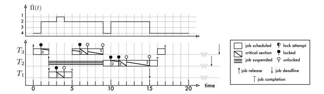
Figure 2.34: SRP schedule of the scenario that results in deadlock under the PIP (Figure 2.32). Similarly to the PCP (Figure 2.33), the SRP avoids deadlock by means of the system ceiling.  $J_{2,1}$  is suspended immediately upon release because its priority does not exceed the system ceiling. At time 9, when  $J_{3,1}$  releases  $\ell_3$ , the priority ceiling is lowered to four and  $J_{2,1}$  becomes eligible to execute.
