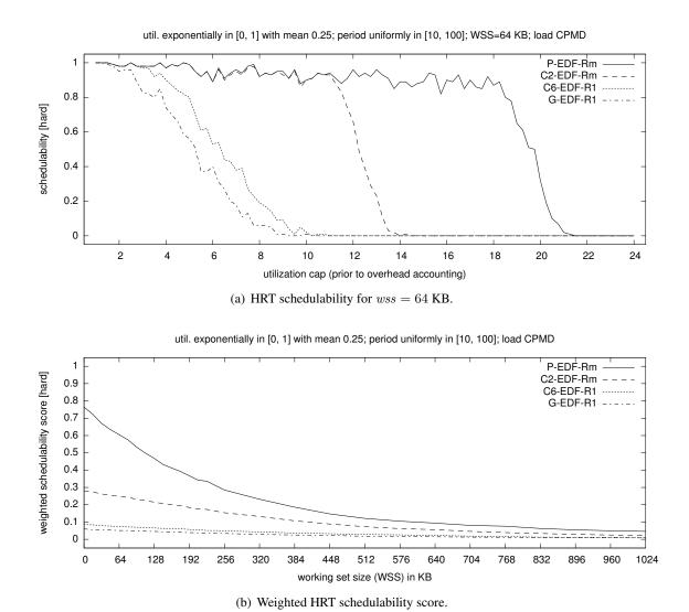
Figure 4.25: Graphs showing (a) HRT schedulability and (b) weighted HRT schedulability score of four EDF-based schedulers with different cluster sizes for medium exponential utilizations and moderate periods.
