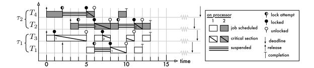
Figure 6.12: P-FP example schedule for m=2 illustrating the FMLP<sup>+</sup> with preemptable critical sections. In this example,  $J_3$  is preempted in the middle of its critical section by  $J_1$  at time 8 when  $J_1$ 's earlier-issued request is satisfied.
