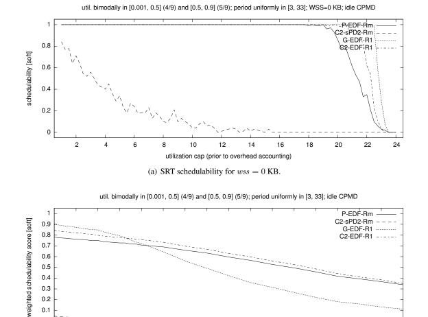
Figure 4.32: Graphs showing (a) SRT schedulability and (b) weighted SRT schedulability score of P-EDF-Rm, C2-EDF-R1, G-EDF-R1, and C2-sPD2-Rm for bimodal heavy utilizations and short periods.
