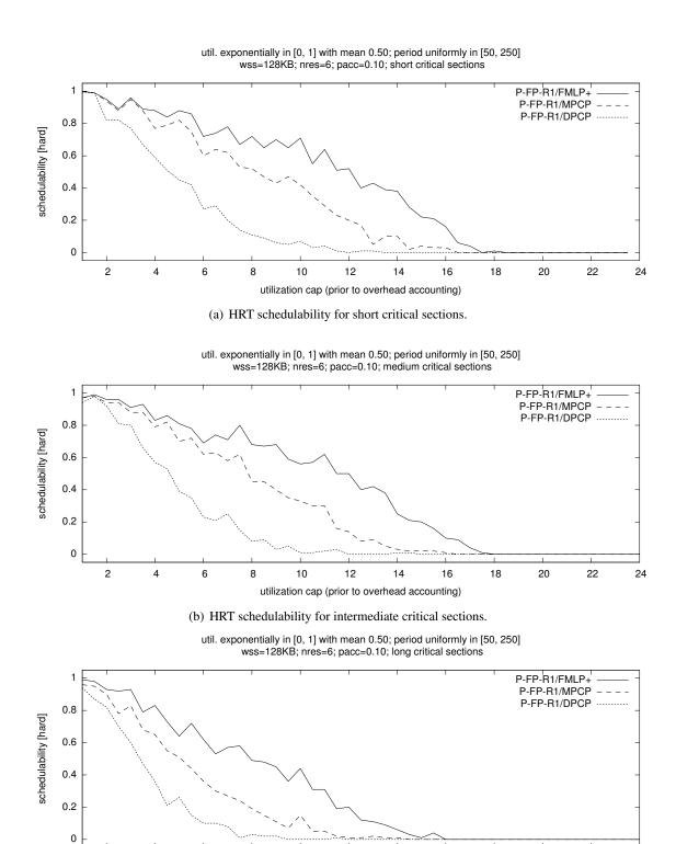
Figure 7.22: Graphs showing HRT schedulability under P-FP-R1 scheduling with the FMLP<sup>+</sup>, the MPCP, and the DPCP for heavy exponential utilizations, long periods,  $n_r = 6$ , pacc = 0.1, and (a) short, (b) intermediate, and (c) long critical sections.
