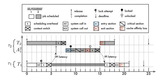
Figure 7.7: Schedule illustrating locking-relate overheads that arise under the DPCP is based on the RPC model, the requesting job must first issue a request to its remote agent, which requires kernel support and hence incurs system call overhead. The remote processor is notified of the pending request with an IPI. Since IPIs are not delivered instantaneously, the requesting job is further twice delayed by IPI latency (once due to the request, and once due to the response).
