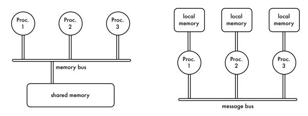
Figure 2.1: Illustration of shared- and distributed-memory multiprocessors. In a shared-memory system, a memory bus enables access to a shared central memory, whereas processors communicate via a message bus that does not allow remote memory access in a distributed-memory system. This dissertation pertains to shared-memory multiprocessors.
