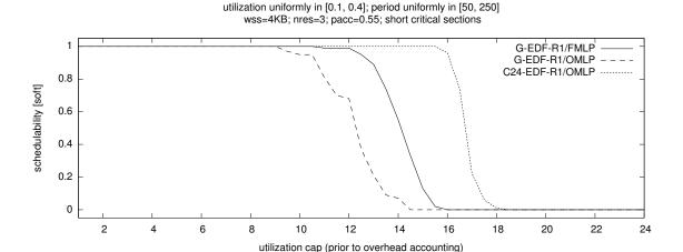
Figure 7.19: SRT schedulability under G-EDF-R1 scheduling with the global FMLP, G-EDF-R1 scheduling with the global OMLP, and C24-EDF-R1 scheduling with the clustered OMLP for medium uniform utilizations, long periods,  $n_r = 3$ , pacc = 0.55 and short critical section lengths.
