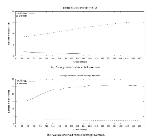
Figure 4.13: Average observed (a) timer tick and (b) release interrupt overhead under C6-aPD<sup>2</sup>-Rm and C6-EDF-Rm. As no job scheduling is required, timer ticks create only little overhead in event-driven schedulers and release ISRs cause only little overhead in quantum-driven schedulers.
