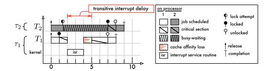
Figure 7.1: Schedule illustrating locking-related transitive interrupt delays. When a resource-holding job is stopped by an interrupt service routine (ISR), any jobs waiting for the resource to be released are transitively delayed as well. In the depicted example, job  $J_1$  on processor 1 is stopped by an ISR during [2–4]. This increases  $J_1$ 's effective request length, which causes job  $J_2$  on processor 2 to incur additional s-blocking.
