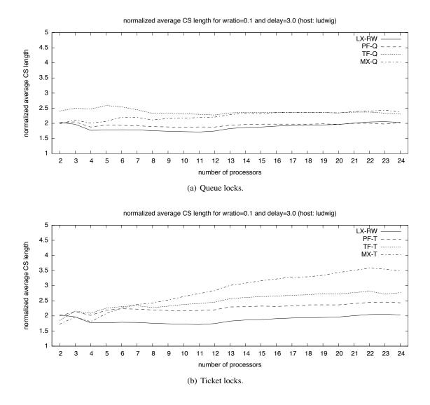
Figure 7.10: Average critical section length as a function of the number of contending processors, grouped by implementation technique with Linux as a baseline. See Table 7.2 for a list of the considered lock types.
