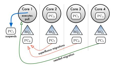
Figure 3.1: Example of unneeded migrations caused by Linux's pull operation. When process  $PC_1$  suspends, process  $PC_5$  must be pulled from runqueue  $RQ_4$  to runqueue  $RQ_1$  so that it can be dispatched next. However, since Linux's pull operation examines remote runqueues in order of increasing indices, two unneeded migrations are triggered as well.
