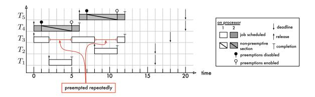
Figure 3.5: Illustration of repeated, eagerly enacted preemptions. Five jobs are scheduled under G-EDF on m=2 processors. Job  $J_3$  is preempted repeatedly even though it is among the two highest-priority ready jobs. This example demonstrates that jobs may be preempted repeatedly if preemptions are enacted eagerly.
