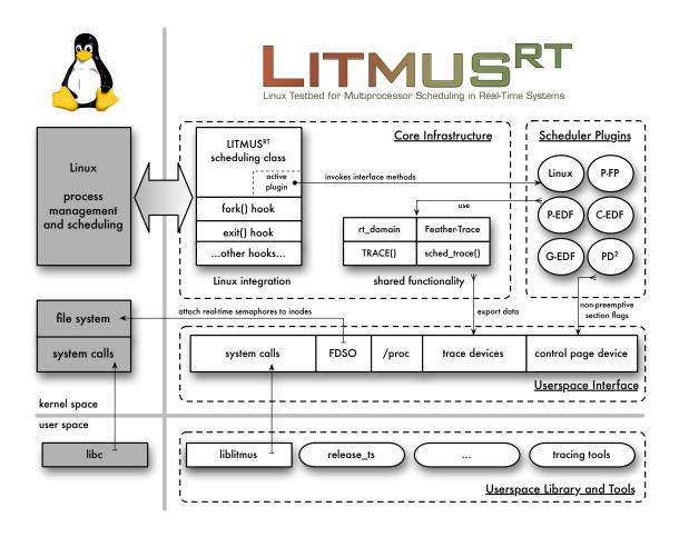
Figure 3.3: Diagram of the structure of LITMUS<sup>RT</sup>, which is comprised of four main components.
