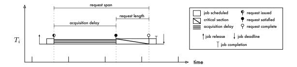
Figure 2.26: Illustration of the phases of a request. A job must wait by either spinning or suspending while it incurs acquisition delay.
