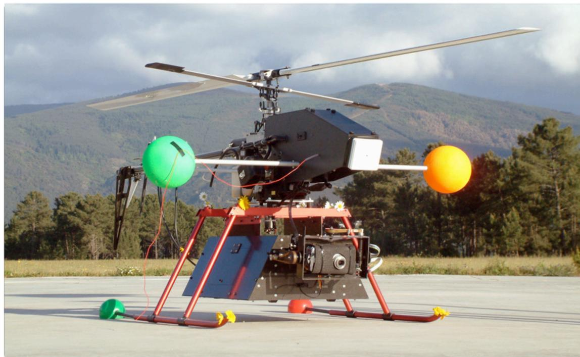
*MARVIN Mk II: unmanned autonomous vehicle (UAV)*
