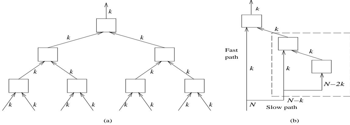
Figure 3: Two approaches for implementing  $Acquire(N, k)$ .  $Release(N, k)$  is implemented analogously. Each arrow represents a set of processes. Solid boxes represent  $Acquire(2k, k)$ . (a)  $Acquire(8k, k)$  in a tree. (b) Using a “fast path” to split off  $k$  processes. The dotted box represents  $Acquire(N - k, k)$ . One approach for implementing  $Acquire(N - k, k)$  using nested fast paths is depicted for  $N = 4k$  (so  $N - 2k = 2k$ ).
