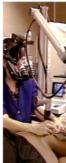
Fig. 4. Left: human subject experiment on January 5, 1996. During preliminary exploration, the physician uses the AR system. The mechanical tracker for the transducer is visible in the foreground. Center and right: stereo view within HMD. The system was not used for the actual intervention.
