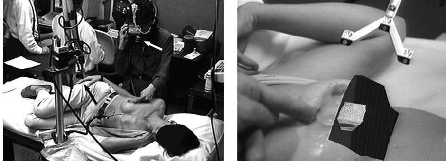
Fig. 1. Left: human subject experiment on April 7, 1995. The physician, wearing a HMD (marked by white arrow) examines the subject's right breast. The black arrow points to the ultrasound transducer attached to the mechanical arm for precise 6 degree-of-freedom tracking. Right: view inside HMD during the experiment in Fig. 1. The synthetic pit contains several ultrasound slices; the frontmost slice is a cross-section through a cyst (dark spot). The physician's finger points to the cyst as she perceives it via tactile feedback. The Y-shaped arm holds landmarks used to maintain correct registration between synthetic imagery and the patient.
