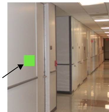
Figure 1: An Example of depth ambiguity in an OIV/AR mockup. In this display, the location (in depth) of the rendered square (marked with an arrow) is ambiguous. Is it on the surface in the hallway, to right of the near room? In the near room? In the far room? There is no definite way to tell because 2D-planar projections of 3D space can be ambiguous.
