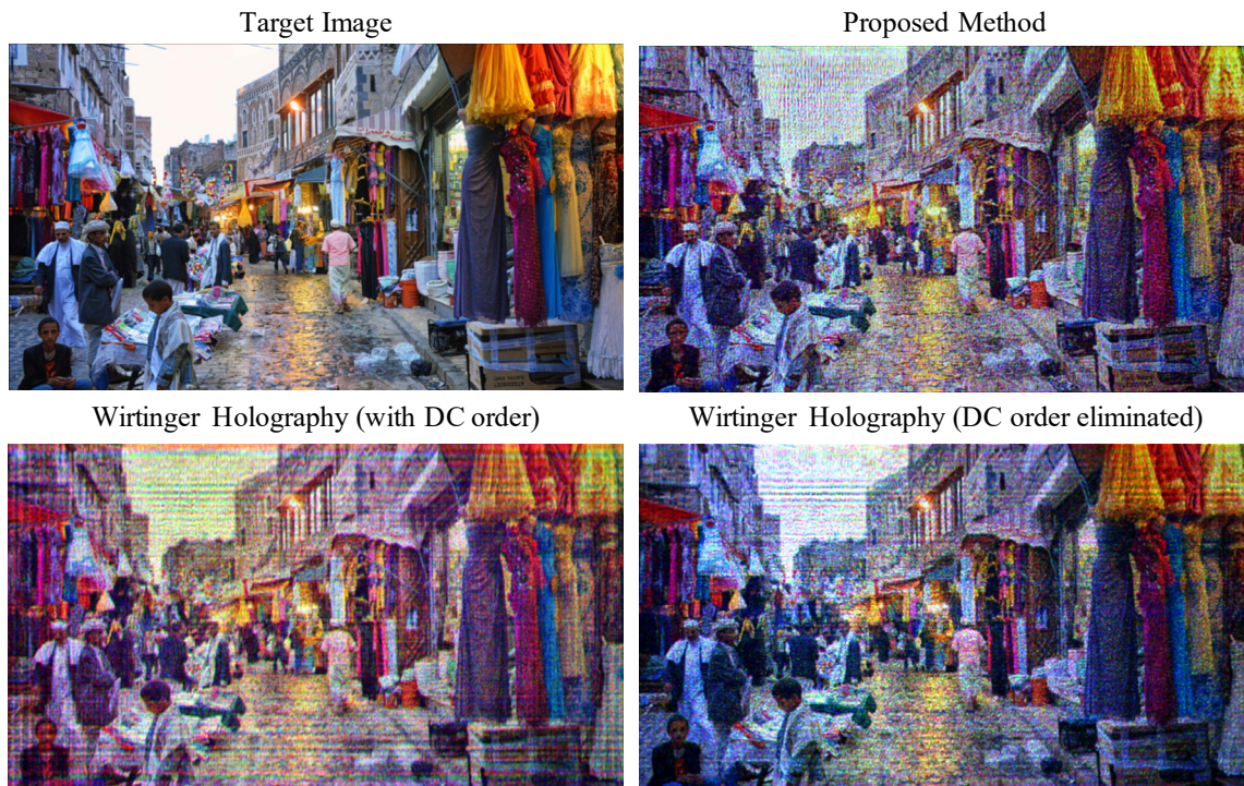
Fig. 5. The display capture for Wirtinger holography with DC order removed shows several dark lines across the image. The proposed phase retrieval method effectively removes observable instances of these lines.
