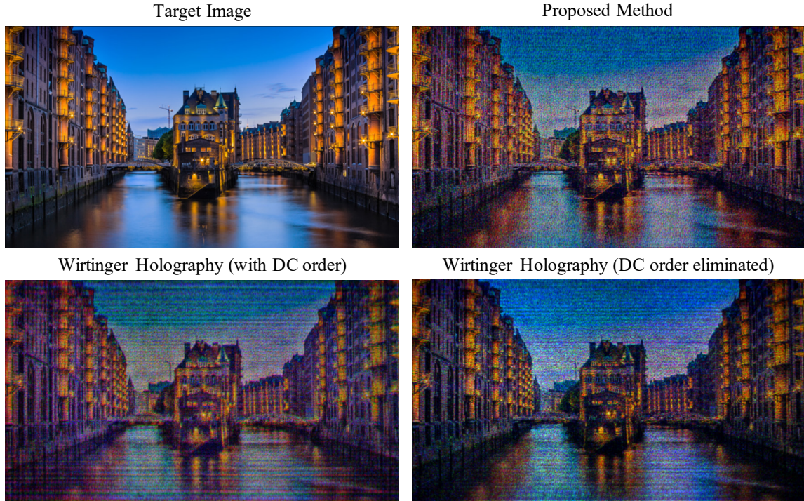
Fig. 4. The proposed method outperforms prevailing phase retrieval methods. If we observe the centre of the display capture using Wirtinger holography with DC order removed, we find several large noisy green pixels alongside visible dark lines across the scene. The proposed method mitigates these streaks and noisy green pixels. Laser speckle is reduced to a much finer resolution with a lighter intensity.
