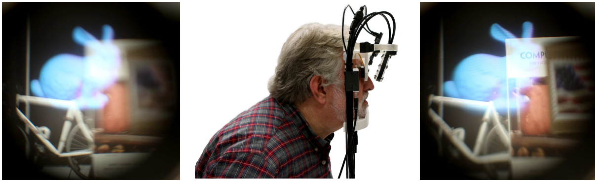
FIGURE 9. (Left) The view of both real and virtual imagery for a presbyopic user with distant vision – with the accommodation depth fixed at 7 m – on a conventional AR HMD. The virtual bunny is at a mid-distance (1 m) together with the stamp (0.25 m), text book (1 m) and bicycle (5 m) arranged at near, medium and far distances respectively. Notice that both the real and virtual imagery appears blurred to the user as none of the objects are in the presbyopic user's accommodation range. (Middle) A presbyopic user with near-zero accommodation range looking through our auto-focus AR eyeglasses. Our prototype AR eyeglasses are capable of providing well-focused imagery of both real and virtual objects at all depths by independently adjusting for the user focus for viewing both real world and virtual imagery from the internal display, based on the user's current eye accommodation state. (Right) The well-focused view of both real and virtual objects of the same scene on our auto-focus AR eyeglasses, due to independent focus adjustments for both real and virtual. Notice that the letters on the textbook at the mid-distance (1 m) are in sharp focus, as well as the virtual bunny, which also is set to appear at the mid-distance.
