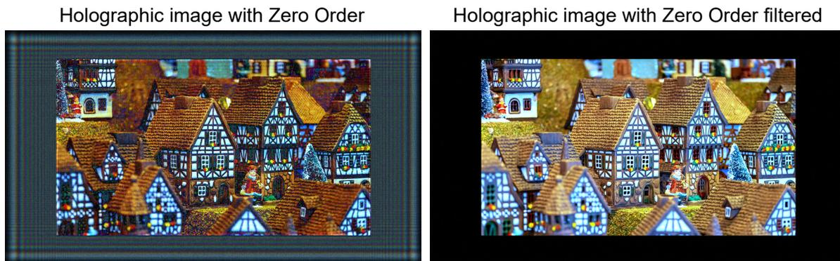
Fig. 8. Simulation of zero order filtering: Filtering the Zero order light improves the holographic image quality significantly.
