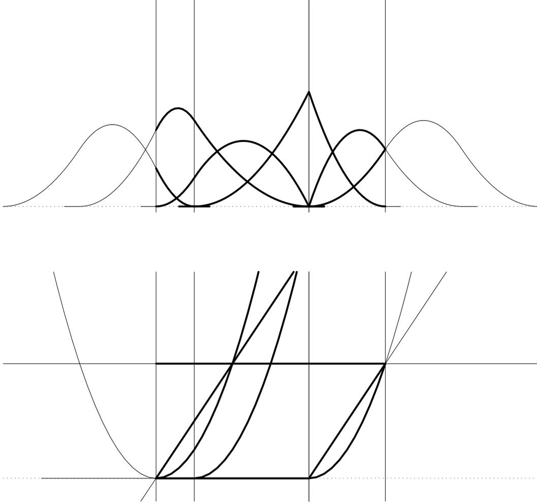
Figure 5.4 (a) The six quadratic B-splines for the case of one simple and one double interior knot; and
