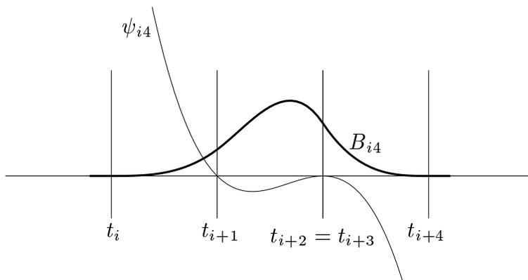
Figure 5.1  $B_{i4}$  and  $\psi_{i4}$ ; note the double knot
