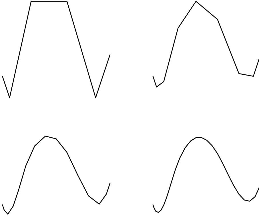
Figure 11.2 The control polygon of Fig. 11.1 and three midpoint refinements.
