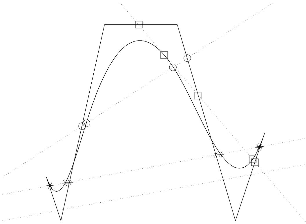
Figure 13.1 A cubic spline, its control polygon, and various straight lines intersecting them. The control polygon *exaggerates* the shape of the spline. The spline crossings are bracketed by the control polygon crossings.
