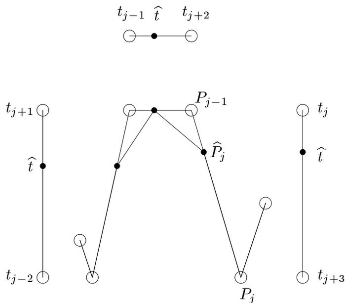
Figure 11.3 Insertion of  $\hat{t} = 2$  into the knot sequence  $\mathbf{t} = (0, 0, 0, 0, 1, \mathbf{3}, 5, 5, 5, 5)$ , with  $k = 4$ .
