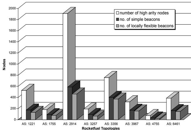
Fig. 5. Histogram of beacon set sizes yielded by different algorithms for the Rocketfuel topologies.
