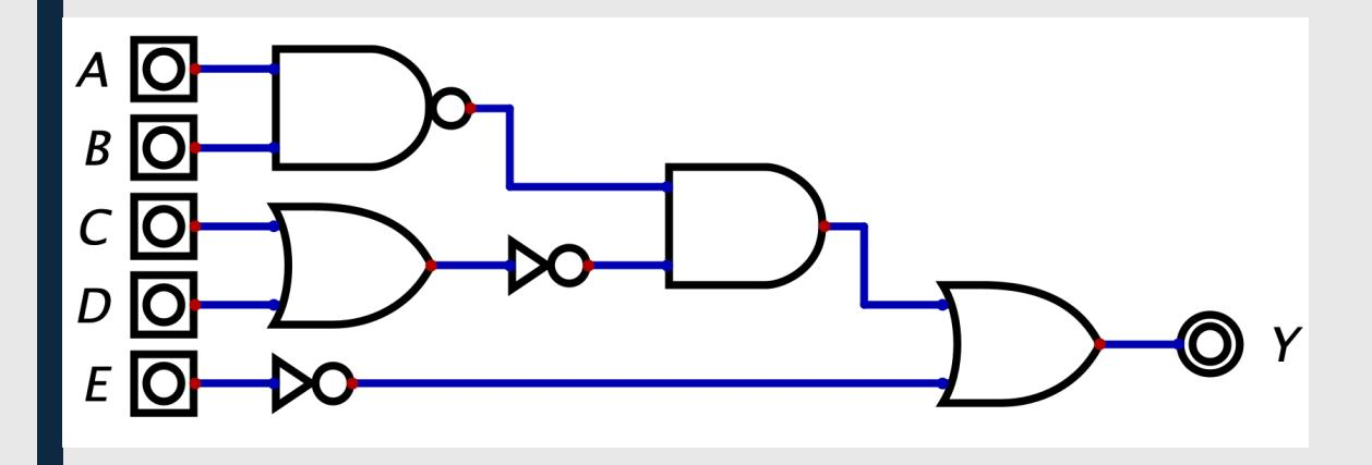
$$Y = (\overline{AB})\overline{(C+D)} + \overline{E}$$
