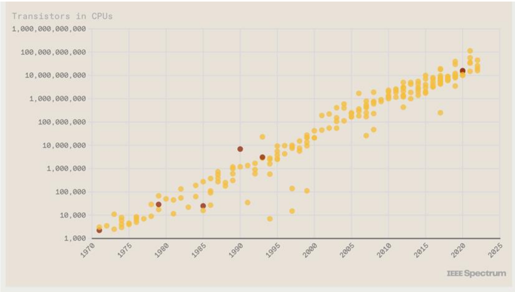
Number of Transistors in CPUs over Time
