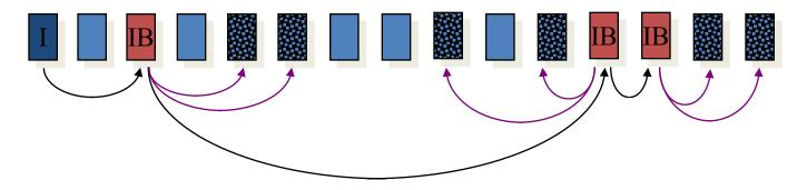
Multilevel indirect blocks (IB\*IB\*...)
