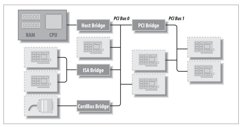
Figure 12-1. Layout of a typical PCI system
