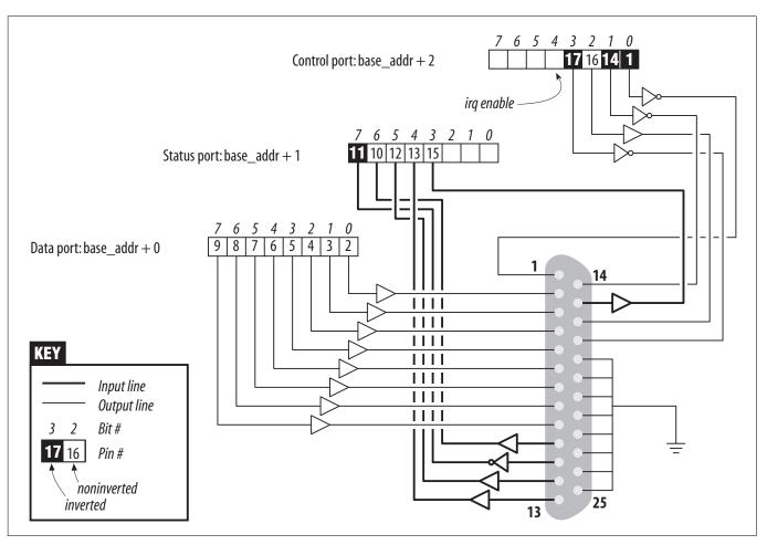
Figure 9-1. The pinout of the parallel port
