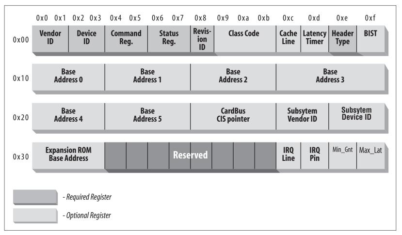
Figure 12-2. The standardized PCI configuration registers
