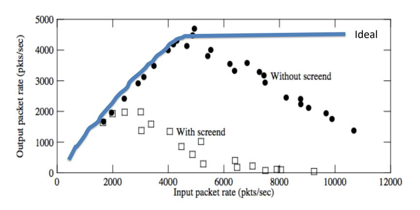
Fig. 2. Forwarding performance of unmodified kernel.
