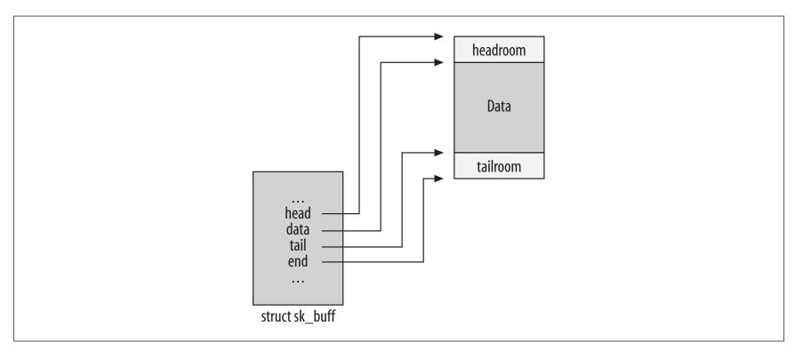
Figure 2-2. head/end versus data/tail pointers
