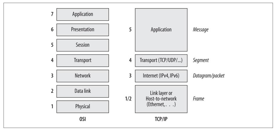
Figure 13-1. OSI and TCP/IP models
