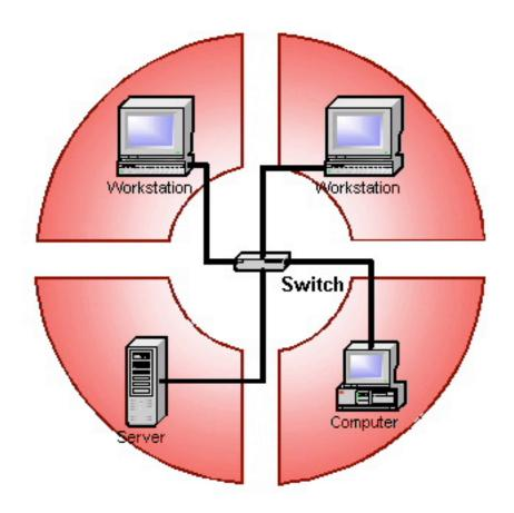
**Switched Full Duplex Ethernet:** 1 collision domain per node. Use of switch. No possibility of collisions. Deterministic.
