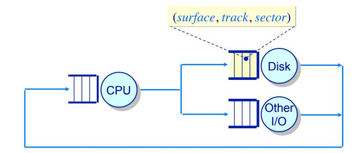
The OS maximizes disk I/O throughput by minimizing head movement through *disk head scheduling*
