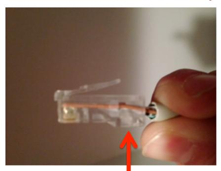
End has a spikey-thing that presses into the wires, holding end on and wires in place
