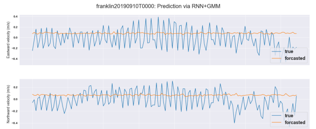
Fig. 4: RNN + GMM prediction performed on the same data collected by Franklin glider in September 2019
