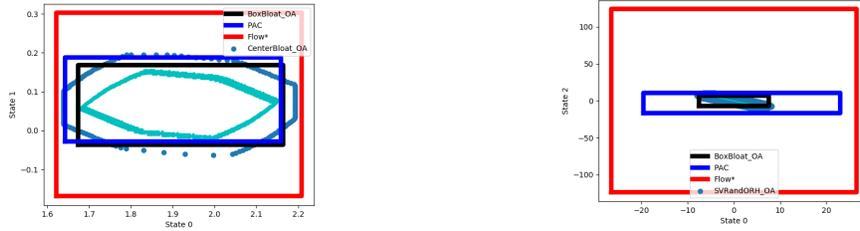
**Figure 2.13: Left:** Over-approximate reachable sets of 5 Vehicle Platoon model. Dirty Blue: Computed using `bloatMean`; Black: Computed using `boxBloat`; Cyan: Random reachable set; Navy Blue: Computed using `modelLearn`; Red: Computed using `Flow*`. **Right:** Over-approximate reachable sets of Spacecraft Rendezvous model. Dirty Blue: Computed using `maxSV`; Black: Computed using `boxBloat`; Cyan: Random reachable set; Navy Blue: Computed using `modelLearn`; Red: Computed using `Flow*`.
