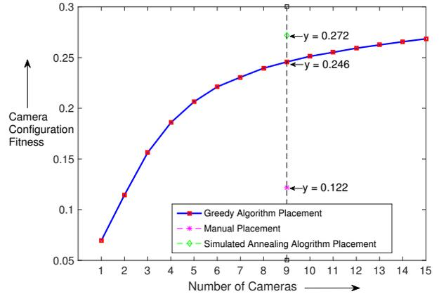
Figure 9: Fitness scores for camera placements using the greedy algorithm, the simulated annealing algorithm, and manual placement.
