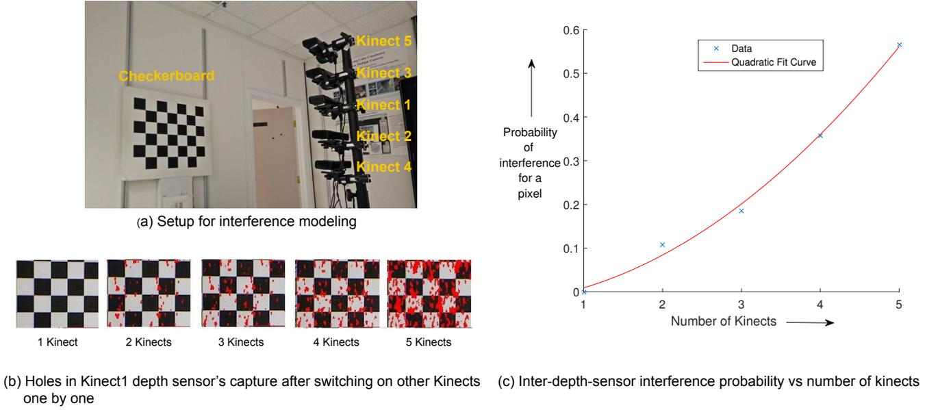
Figure 5: Multiple Kinects setup for interference modeling.
