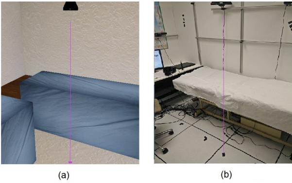
Figure 10: (a) marker position of projected camera center on the floor in the simulation; (b) marker position of projected camera center on the floor in the capture room. The pink lines represent the optical axes of the corresponding cameras, extended to the marker on the floor.
