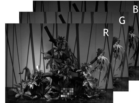
raw-RGB represents the physical world's SPD "projected" onto the sensor's spectral filters.
