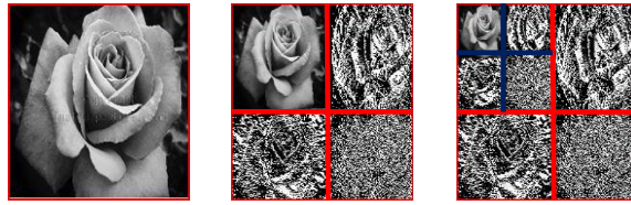
Fig.6 1-level and 2-level haar operation on a gray scale image
