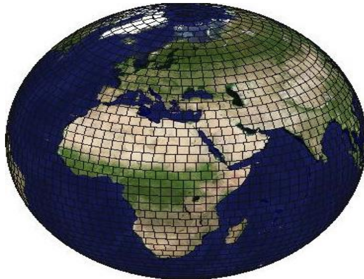
Figure 2: Discretization of Earth into 3186 bins [2]
