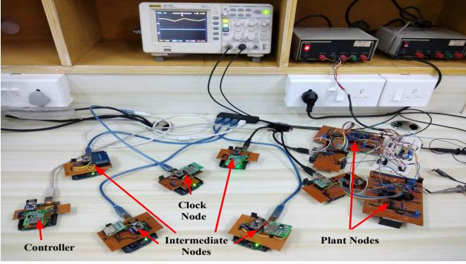
Figure 3: The CPS testbed consisting of a control node, four intermediate nodes and two physical plants.
