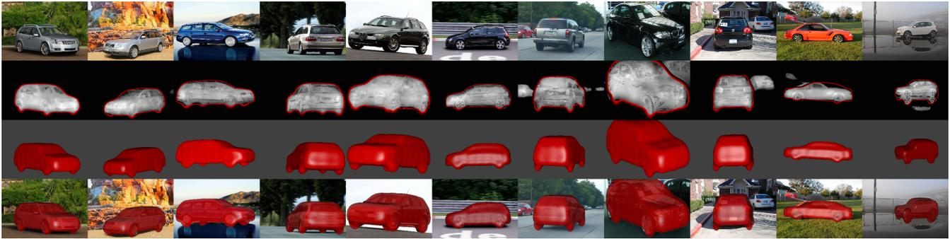
Fig. 22: More results of monocular 3D Shaping. The first nine columns show successful reconstructions from different viewpoints. The next-to-last column shows a failed reconstruction with a 180°-flipped viewpoint. The last column exhibits another failure due to strong reflection from the wheel.
