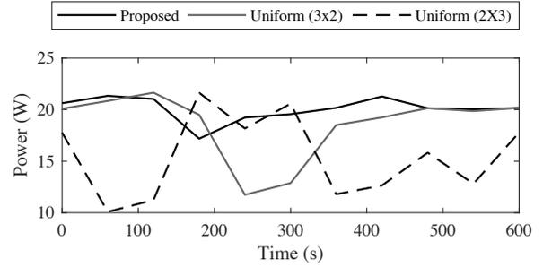
Fig. 8: Power generation over solar irradiance profiles for 60 cell array on a semisphere surface. Mean power is 20.04 W, 18.45 W, and 15.26 W, respectively for three cases.
