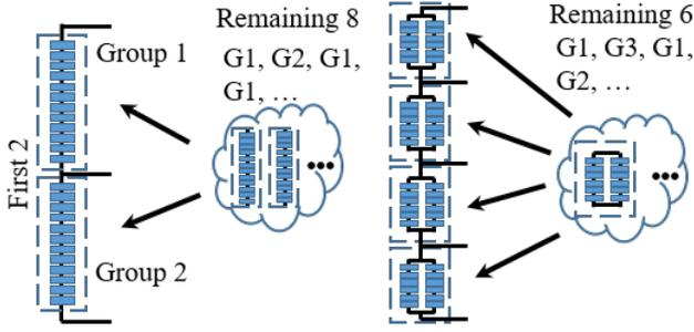
Fig. 6: Flexibility according to the size of atomic unit for reconfiguration.  $12 \times 1$  (left) and  $6 \times 2$  (right).
