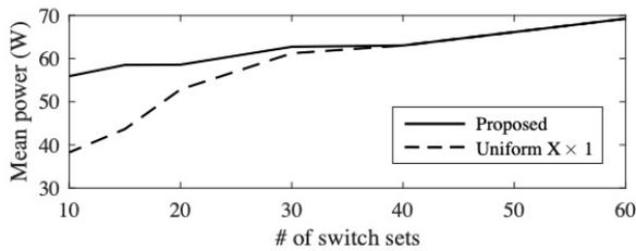
Fig. 10: Trade off between the number of reconfiguration switch sets and the power output for the pyramid example.
