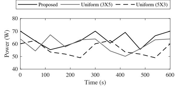
Fig. 7: Power generation over solar irradiance profiles for 120 cell array on a pyramid surface. Mean power is 63.63 W, 59.37 W, and 55.41 W, respectively for three cases.
