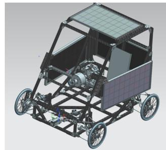
Fig. 1: A custom designed EV with four PV modules.
