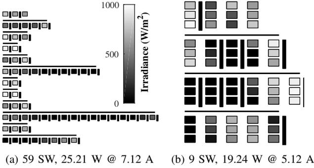
Fig. 5: (a) PV array on a sphere surface with max. number of reconfiguration switches, and (b) reduced number of switches.
