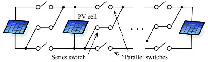
Fig. 3: Reconfigurable PV array architecture.
