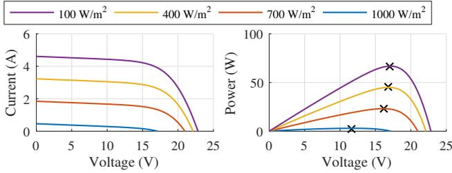
Fig. 2: VI curve of a PV module.
