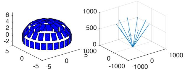
Fig. 4: An example PV array on a sphere surface and 11 light vectors for the motivational example.
