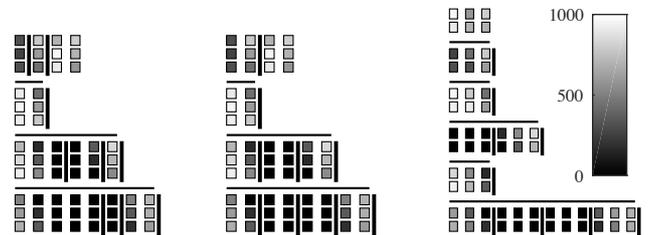
Fig. 9: Switch location and configuration for the first irradiance vector on 60 cell sphere array. Left: proposed, center: uniform  $3 \times 2$ , right: uniform  $2 \times 3$ . Color denotes irradiance in ( $\text{W}/\text{m}^2$ )
