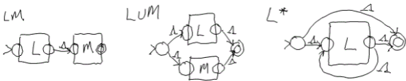
Figure 12.5: Combining machines for languages L and M to make machines that accept LM , L \cup M , or L^* .
