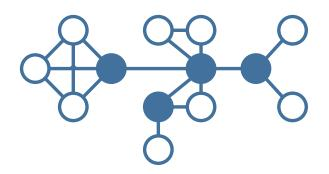
We can determine articulation points using depth-first search. Let  $G_{\pi} = (V, E_{\pi})$  be a depth-first tree of G.
