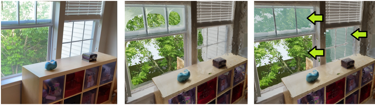
Fig. 1. Left : ground truth image. Before (Middle) and after (Right) audio-augmented rendering of an indoor scene with open and closed reflective surfaces. EchoCNN enhances scene reconstruction through more accurate surface detection, depth estimation, and material classification based on audio-visual reflecting sound and image inputs. Green arrows highlight areas enhanced by our method.
