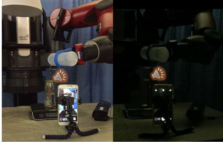
Figure 4.1: Our audio-augmented approach performs weight estimation, overflow detection, and content and container classification in bright environments (left) whereas our audio only based approach can be used in dark and occluded environments (right). Pouring sequences are recorded using either a smartphone or Microsoft Kinect’s built-in microphone array. Training data is generated by assigning digital scale measurements to discrete audio intervals and tested in experiments using Baxter robot and human experimenter pouring sequences. Various contents (water, rice, soda, and milk) and target containers (glass measuring cup, metal cup, Polyphenylsulfone (PPSU) bottle, plastic bottle, plastic cup, and square bowl) were evaluated.
