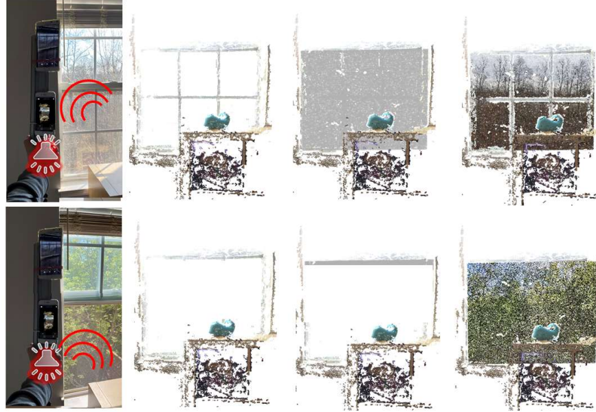
Figure 6.2: Top row : closed window in winter. Bottom row : opened in spring. Column 1 : mobile echoreconstruction prototype; the bottom phone emits pulsed audio and performs a RGB-based 3D reconstruction (live (225) or photogrammetric (144)); the top phone records video. Column 2 : initial reconstruction based on state-of-the-art commercially available Astrivis app. Column 3 : our audio-visual EchoCNN convolutional neural network classifies open or closed surface, depth, and material. Column 4 : semantic reconstruction of the window accounting for EchoCNN inferences.
